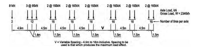
For the EPLL2 truck, transverse wheel spacings for 16 tire groups (8 tire axles) shall be as indicated in Figure 3.8.3.2.3 iii. Transverse wheel spacings for 2 and 12 tire axles shall be similar to those indicated for the CL-W truck in Figure 3.2 of CHBDC. The clearance envelope for the EPLL2 truck shall be assumed to extend 0.3 m on each side beyond the out-to-out width of tires shown in Figure 3.8.3.2.3 iii.
