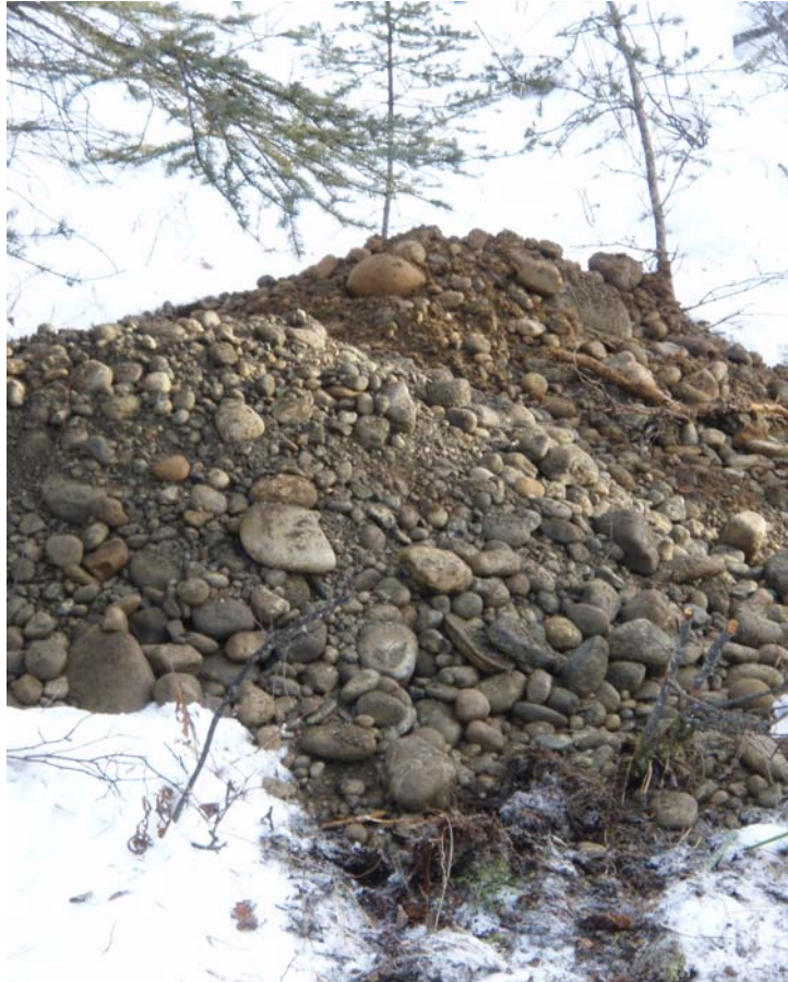
Photo # 5. Pit Run Materials – TP07-19
