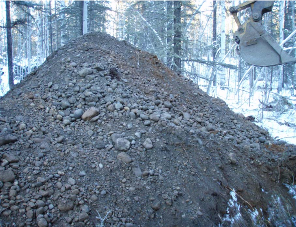
Photo # 1. Pit Run Materials – TP07-06
