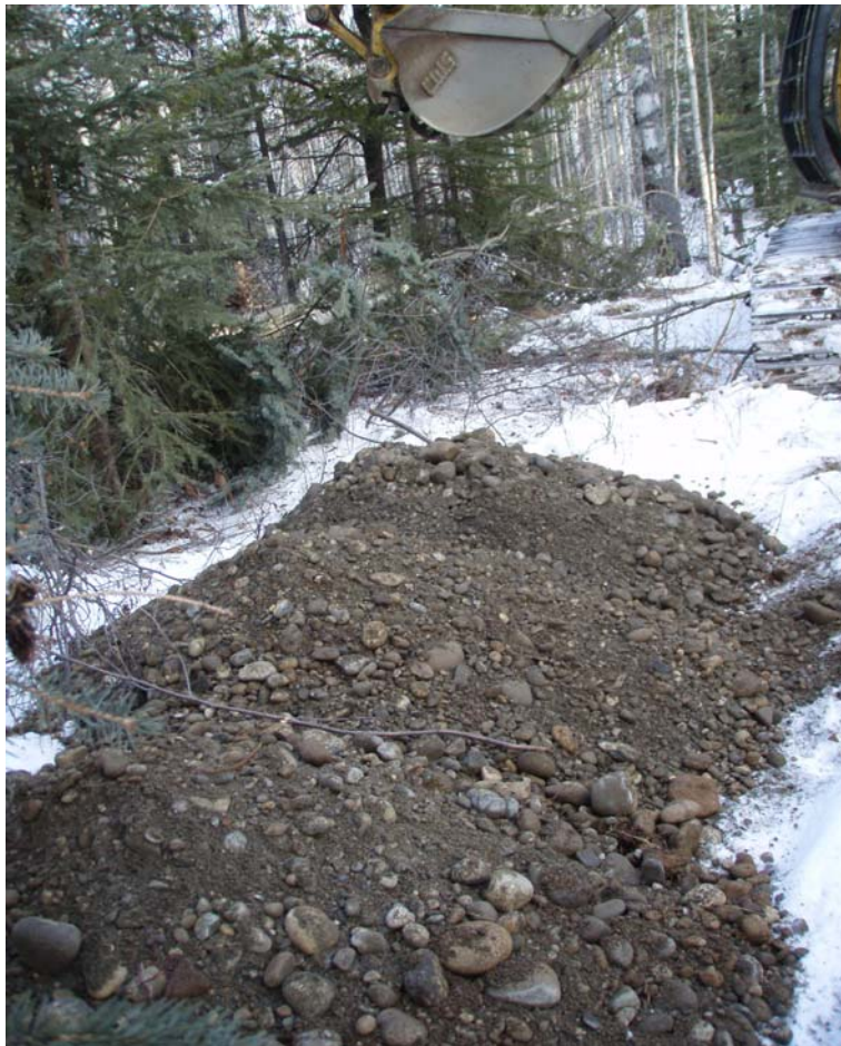
Photo # 11. Pit Run Materials – TP07-26
