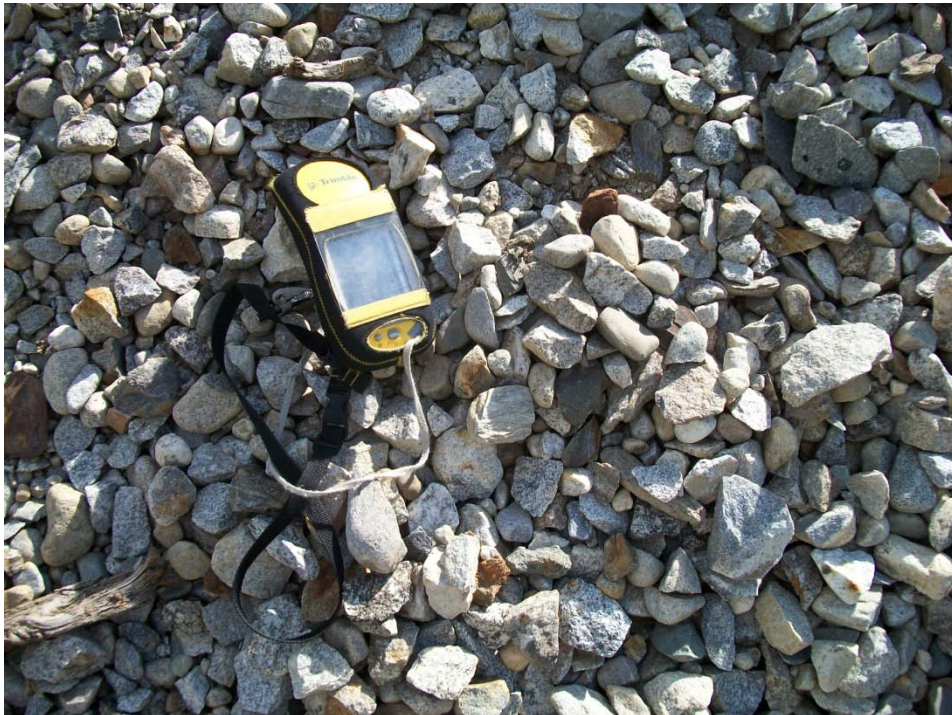
Plate 6. Close up of rain washed aggregate at the base of the crushed stockpile shown in Plate 5. The GPS unit is 22cm.
