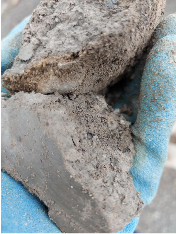
Photo 17 Clay and Silt material at 0.3 m – 1.5 m
