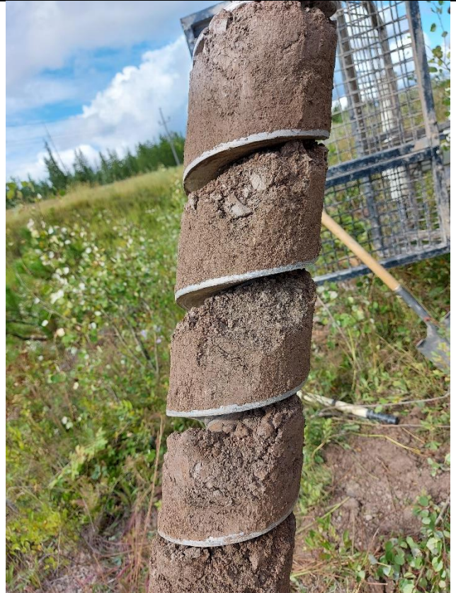
Photo 22 TH21-01 drilled material at approximately 5 m
