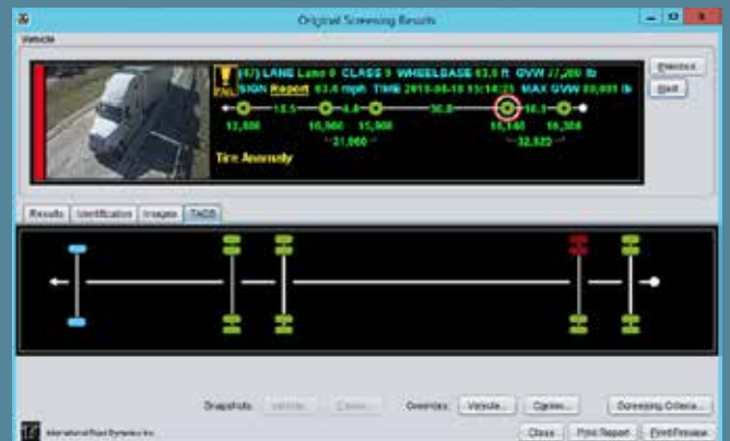
TACS integrates with IRD's operator display to identify tire problems
