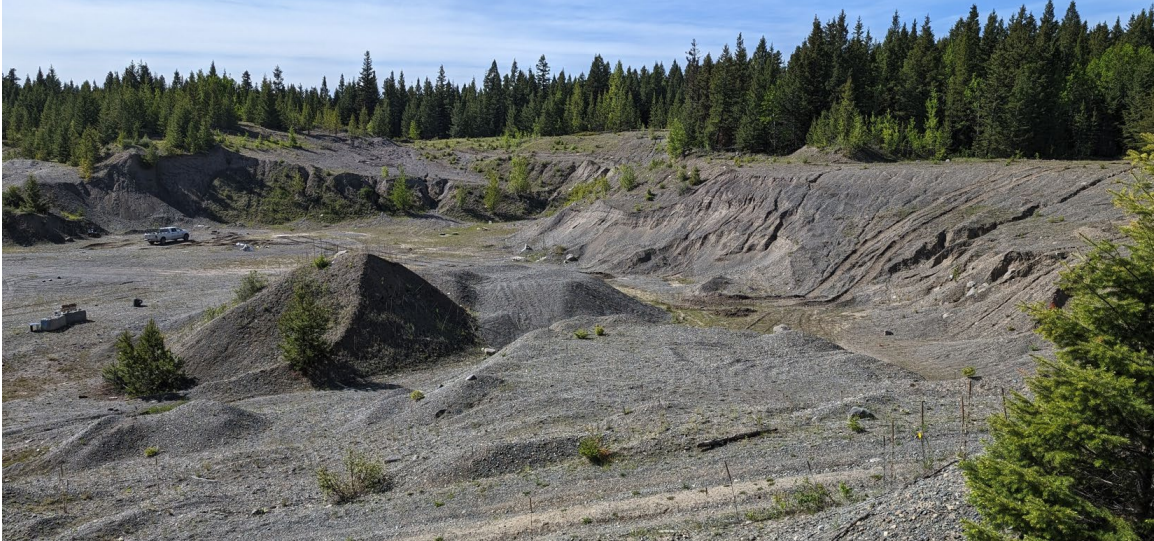
View of secondary mining area, facing south from the western part of pit. Existing stockpiles may have to be relocated. Note the treed area above the pickup truck (TP24-05) contains large quantities of overburden/strippings (2024).
