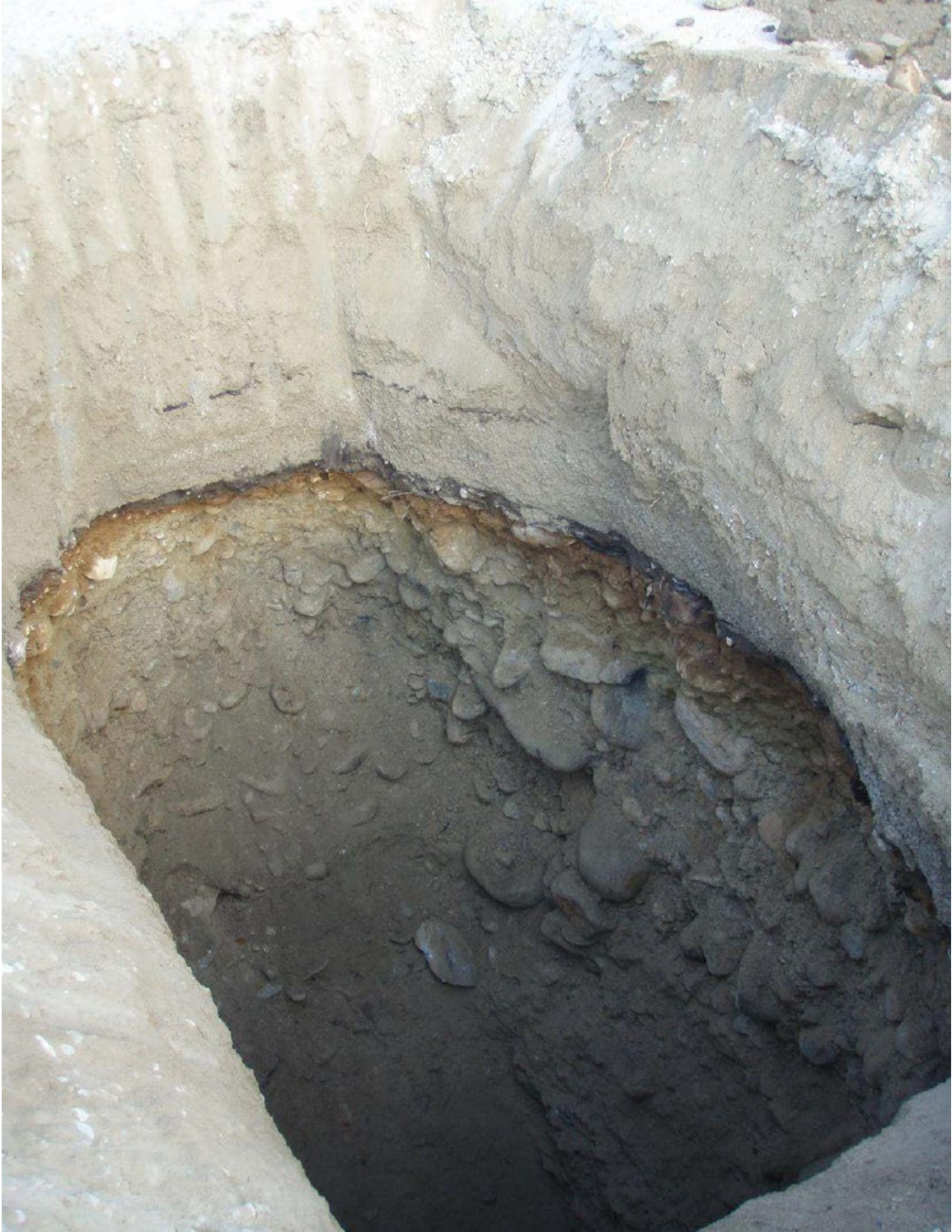
TP14-17 - note layer of material presumed to be asphalt
