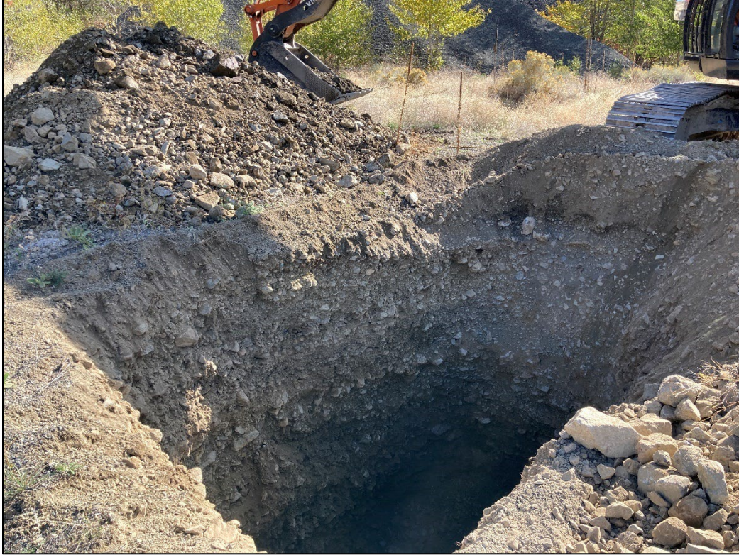
Photo 3 TP21-03 test pit and spoil pile (well-graded gravel) (Oct. 2021).
