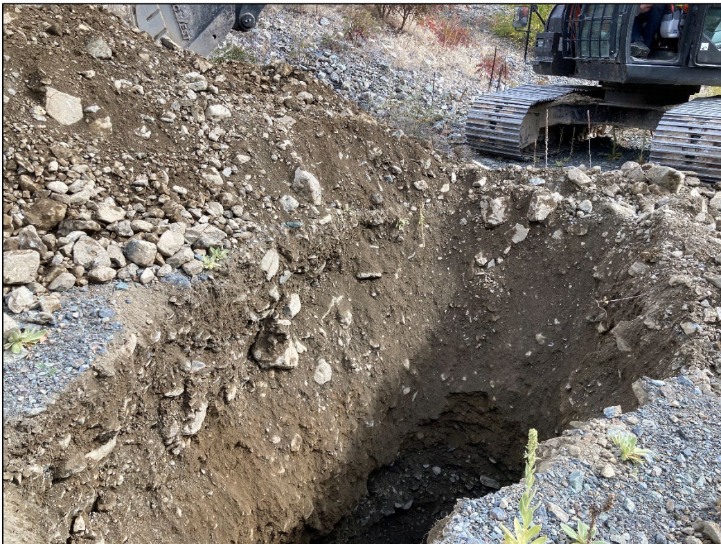
Photo 4 TP21-05 test pit and spoil pile (well-graded gravel). Located at the top of the pit face (Oct. 2021).
