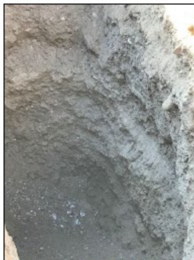
Test Pit 18-03 (coarse gravel to 5.0 metres)
