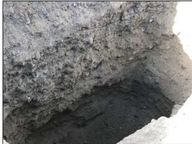
Test Pit 18-05 (gravel to 5.0 metres)
