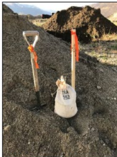
Test Pit 18-01 Spoil (2.1 to 5.0 metres)
