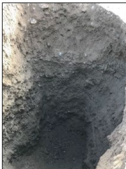
Test Pit 18-06 (gravel to 4.8 metres)
