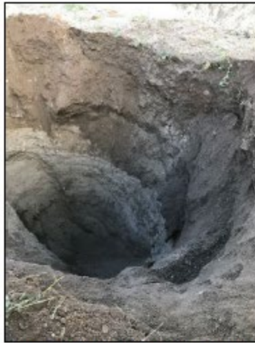
Test Pit 18-01 (fill overlying sand at 2.1metres)
