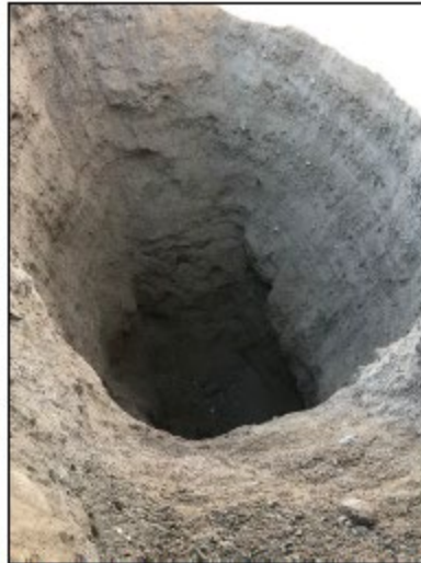
Test Pit 18-02 (medium to fine sand to 5.0 metres)
