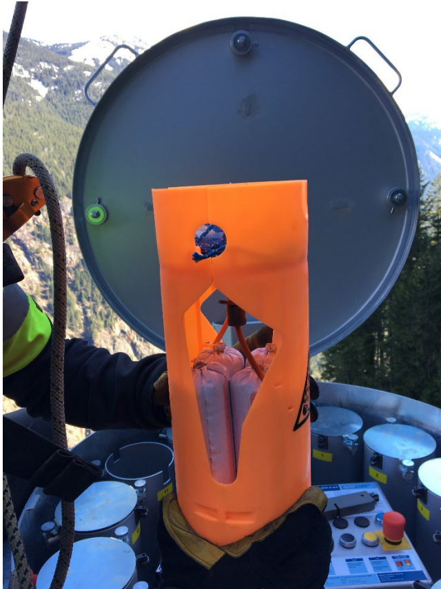
Figure 4. Assembled WAT explosive charge.
