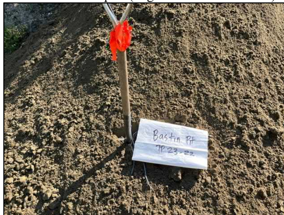
Test Pit 23-22 Spoil (High fines sand 1.8-6.0m)
