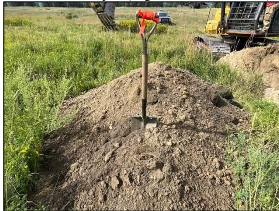
Test Pit 23-10 Spoil (High fines sand 0.1-5.0m)
