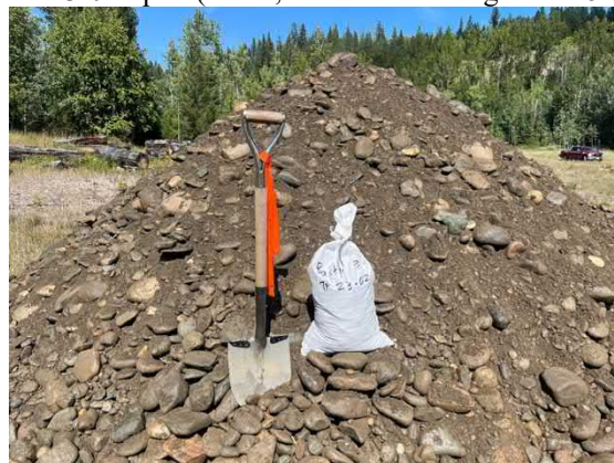
Test Pit 23-02 Spoil (Clean, coarse sand and gravel 0.5-5.2m)
