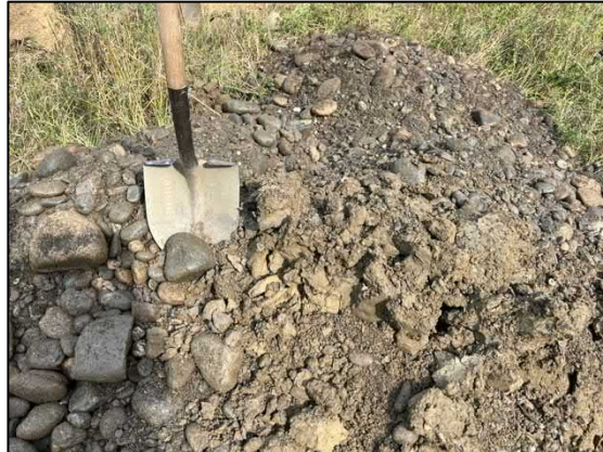
Test Pit 23-17 Spoil (Clay mixed with gravel from 5.5 to 6.0m)
