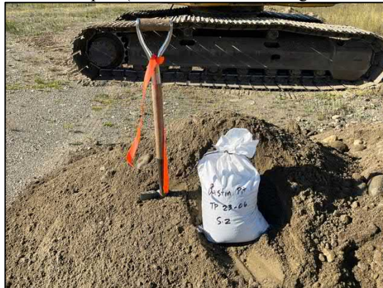
Test Pit 23-06 Spoil (High fines sand 4.2-5.4m)
