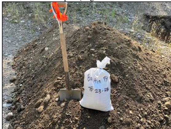
Test Pit 23-23 Spoil (Clean, sandy gravel 0.0-5.0m)
