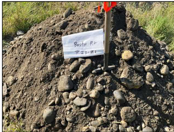
Test Pit 23-21 Spoil (Clean, coarse sand and gravel 2.8-5.5m)
