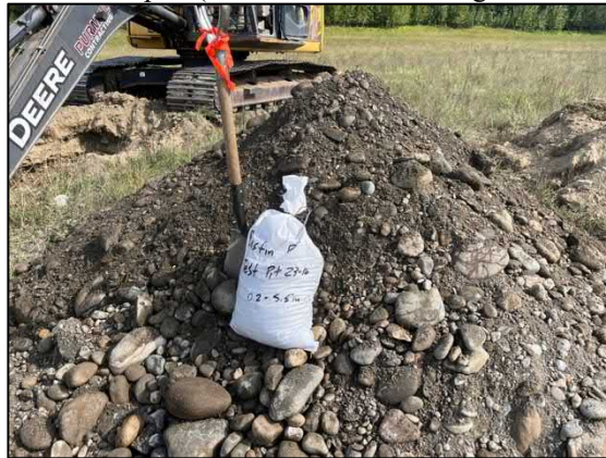
Test Pit 23-16 Spoil (Clean, coarse sand and gravel 0.2-5.5m)
