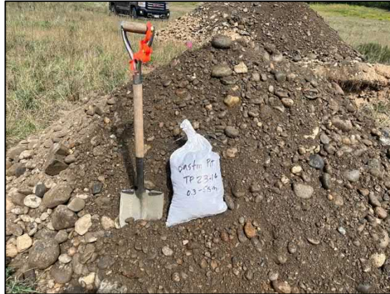
Test Pit 23-14 Spoil (Clean, coarse sand and gravel 0.3-5.6m)
