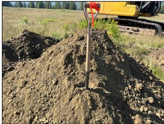
Test Pit 23-09 Spoil (High fines sand 2.8-6.0m)
