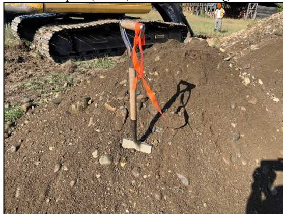
Test Pit 23-08 Spoil (Clean, gravelly sand 4.6-6.0m)
