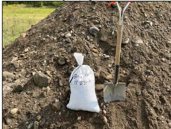
Test Pit 23-11 Spoil (Clean, coarse sand and gravel 1.4-4.0m)
