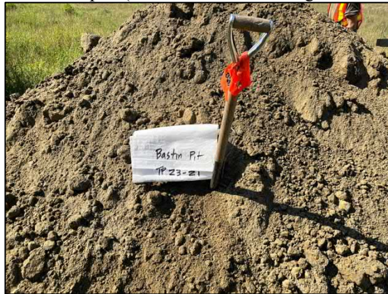
Test Pit 23-21 Spoil (High fines sand 5.5-6.0m)
