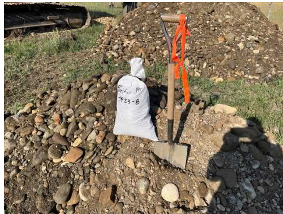
Test Pit 23-08 Spoil (Clean, coarse sand and gravel 0.1-4.6m)
