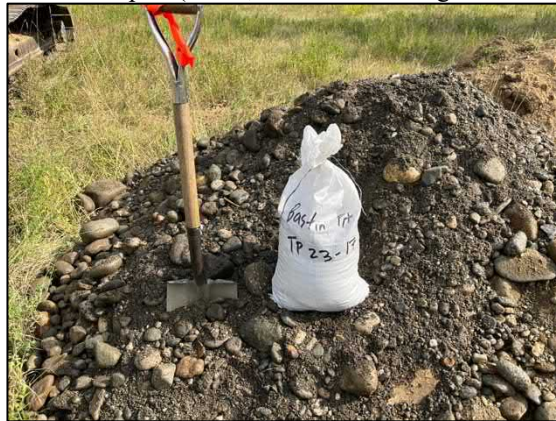
Test Pit 23-17 Spoil (Clean, coarse sand and gravel 0.2-5.5m)
