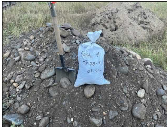
Test Pit 23-18 Spoil (Clean, coarse sand and gravel 0.7-5.0m)
