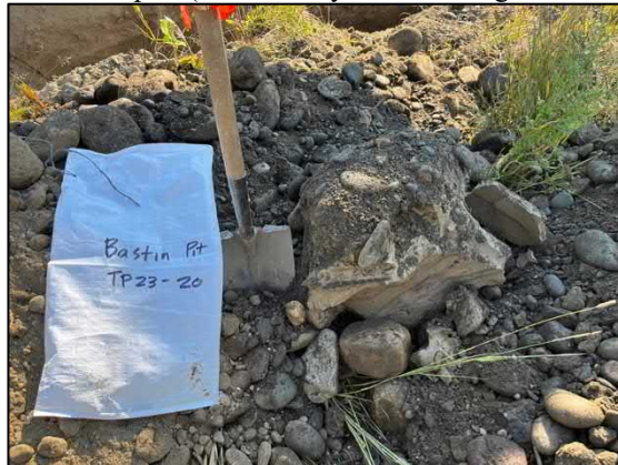
Test Pit 23-20 Spoil (Sand and gravel mixed with large clay lumps 1.2-5.5m)
