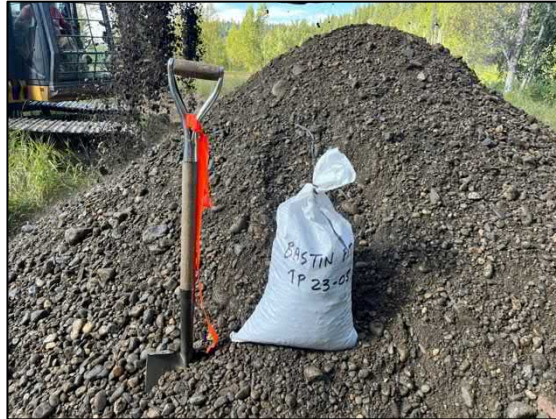
Test Pit 23-05 Spoil (Clean, coarse sand and gravel 2.0-4.5m)
