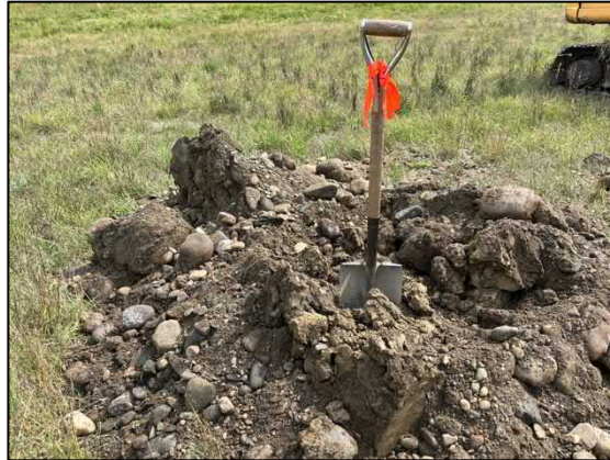
Test Pit 23-12 Spoil (Clay mixed with gravel 4.0-5.5m)
