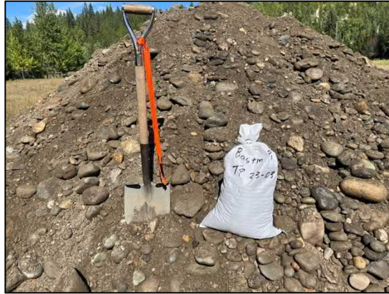
Test Pit 23-03 Spoil (Clean, coarse sand and gravel 0.5-5.2m)
