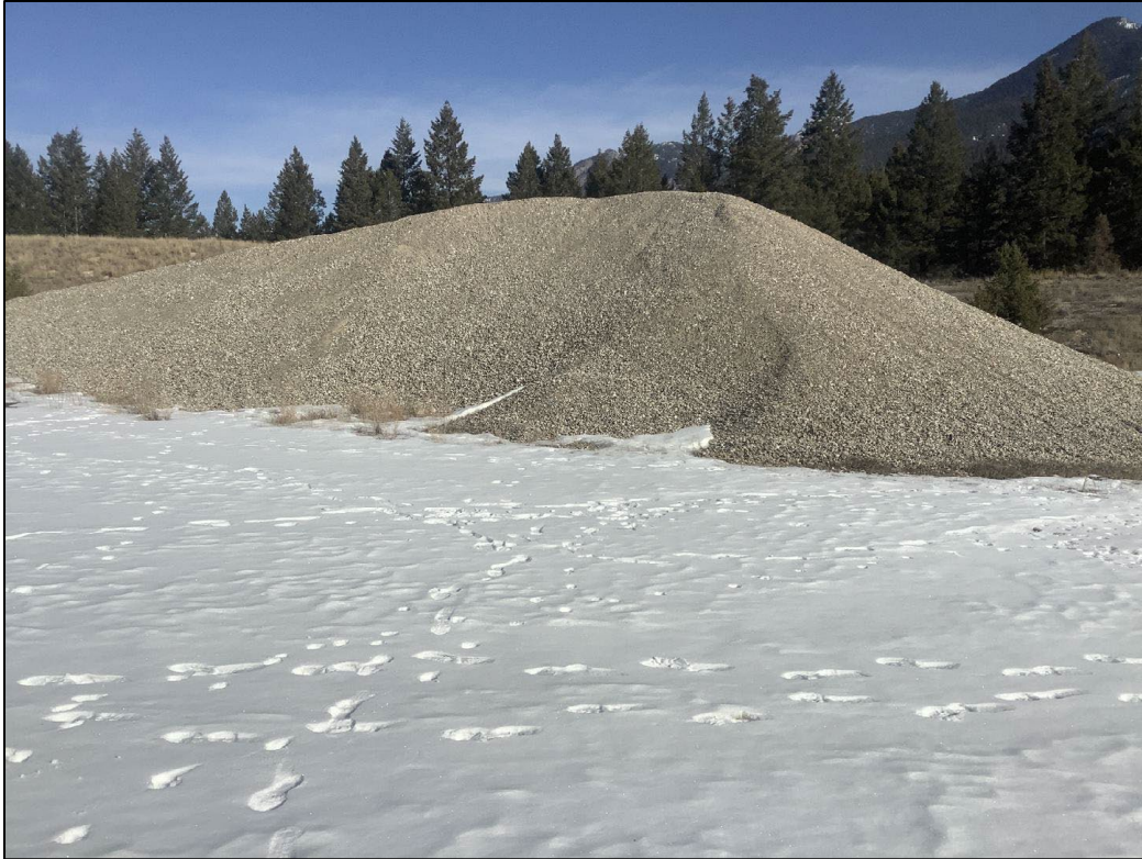
Figure 5 Stockpile 1. Available to use, it is recommended that the material be tested to determine the gradation and if it meets specifications (March 2023).
