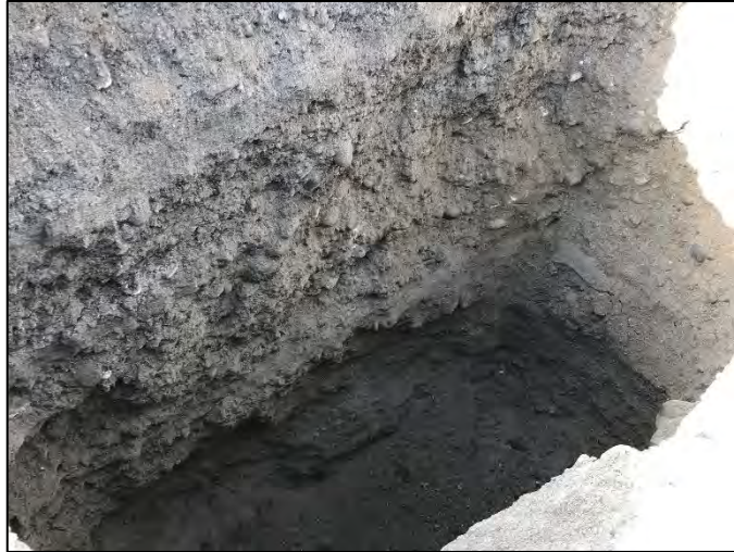
Test Pit 18-05 (gravel to 5.0 metres)
