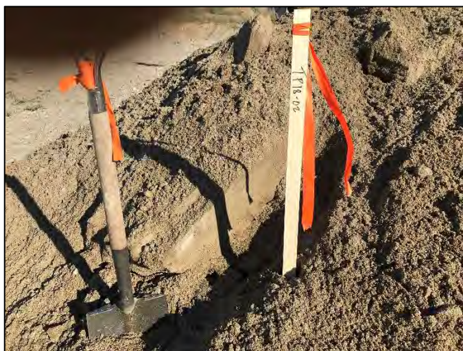
Test Pit 18-02 Spoil ( \text{SM}^3 between shovel and stake)
