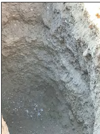
Test Pit 18-03 (coarse gravel to 5.0 metres)
