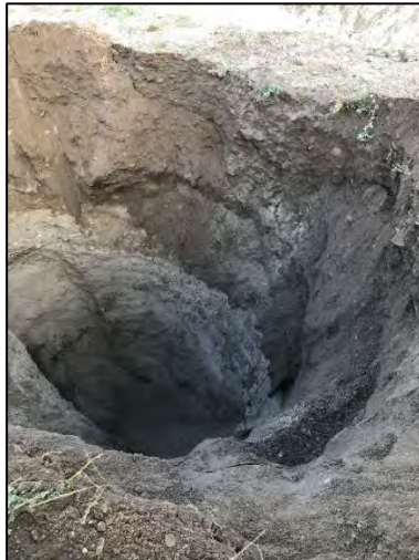
Test Pit 18-01 (fill overlying sand at 2.1 metres)
