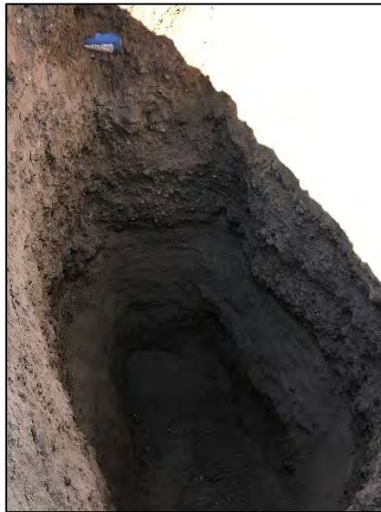
Test Pit 18-11 (sandy gravel underlain by sand at 3.5 metres, minor fill at top of photo)
