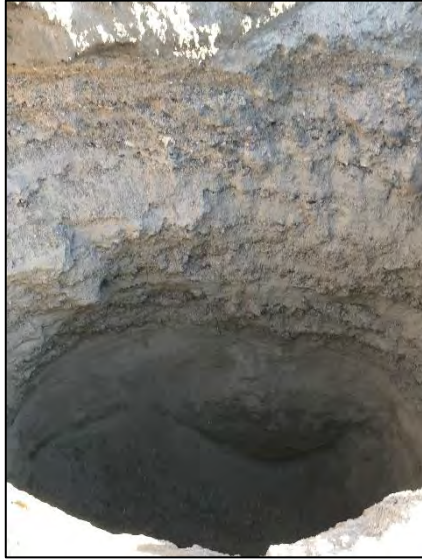
Test Pit 18-13 (Sand underlain by fine sand at 3.2 metres)
