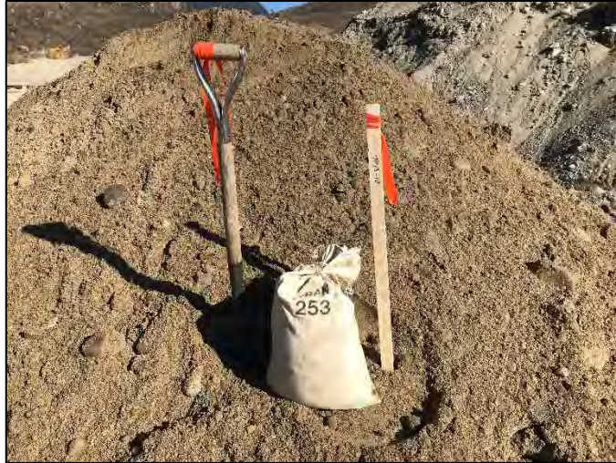
Test Pit 18-10 Spoil (0.0 to 4.5 metres)
