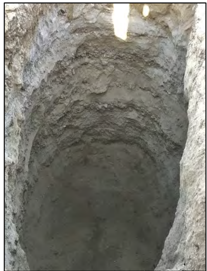
Test Pit 18-14 (sand underlain by fine sand at 3.0 metres)
