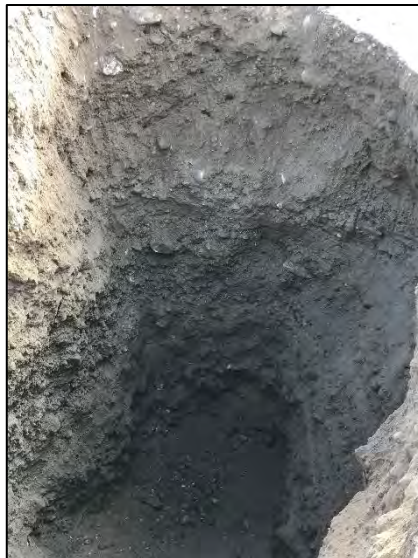
Test Pit 18-06 (gravel to 4.8 metres)
