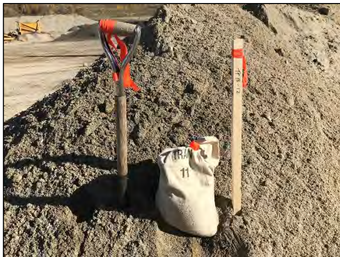
Test Pit 18-12 Spoil (0.0 to 2.5 metres)
