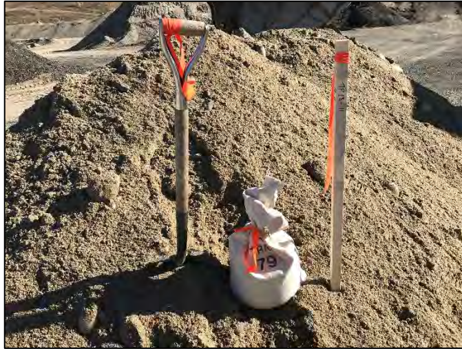
Test Pit 18-11 Spoil (sand from 3.5 to 5.0 metres)
