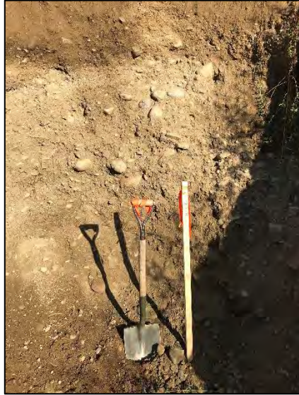
Test Pit 18-17 (fill overlaying gravel at 1.0 metres)
