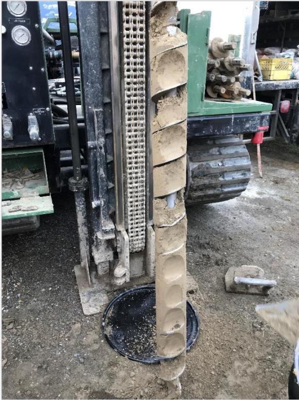
Photograph 5 –Solid stem auger sample showing typical silty SAND encountered on Site. MW18-A1-03.
