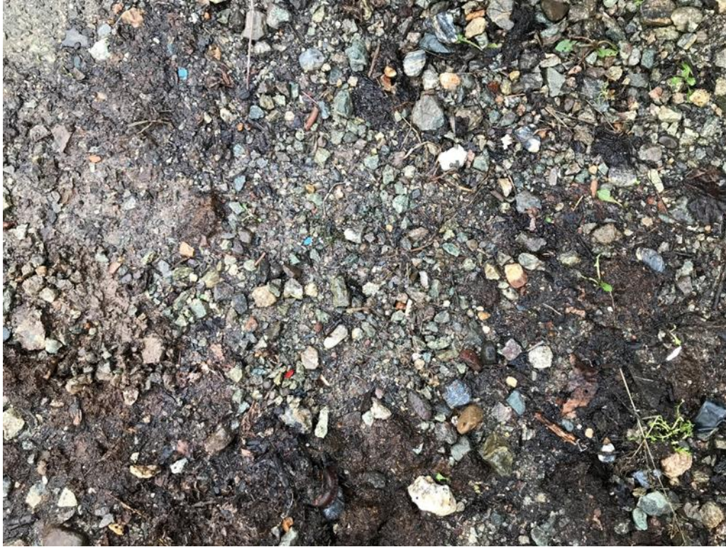
Photograph 7 – Shallow soils were observed to contain various paint flakes and small metals debris throughout the salvage yard.
