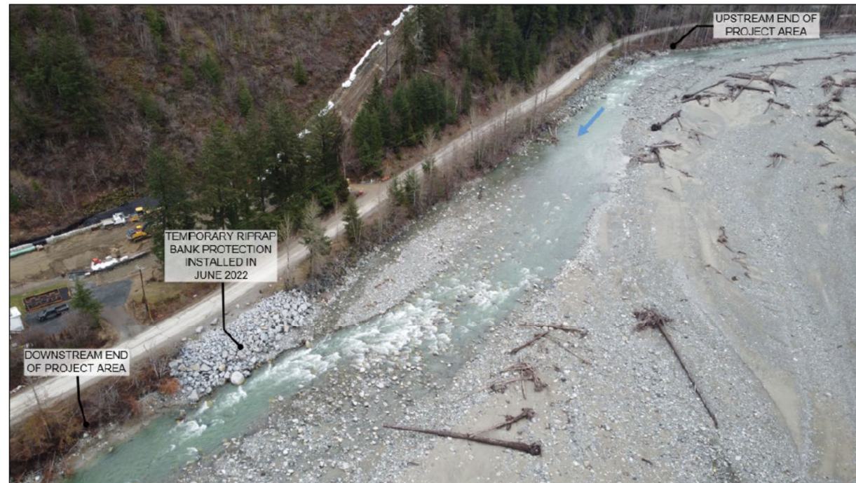
Figure 2-1 (Left) Looking north at temporary riprap mitigation post-construction (Feb 23, 2023). (Right) Looking west at a temporary mitigation design markup prior to construction (March 31, 2022). Both photos are described further in the BGC hydrotechnical report (July 17, 2023).
