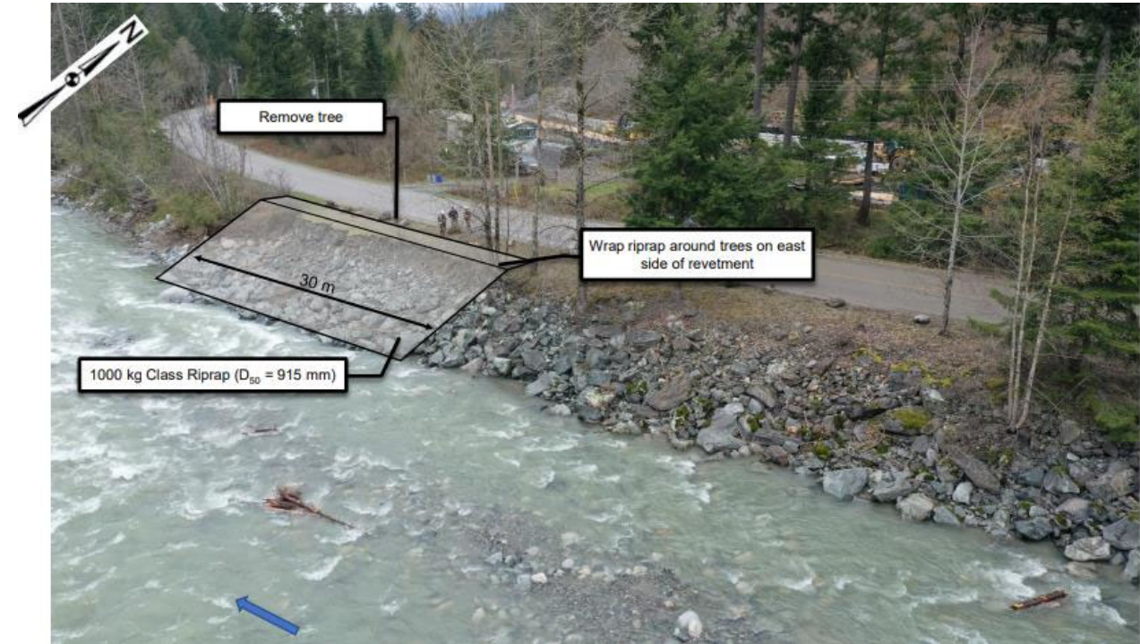
Figure 2-1 (Left) Looking north at temporary riprap mitigation post-construction (Feb 23, 2023). (Right) Looking west at a temporary mitigation design markup prior to construction (March 31, 2022). Both photos are described further in the BGC hydrotechnical report (July 17, 2023).
