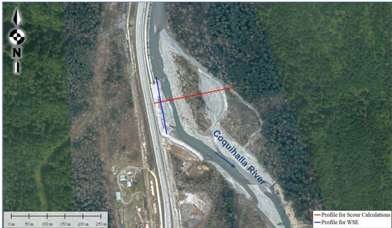
Figure 2-1 Location of hydraulic parameter estimation. WSEs, flow velocity and flow depth were estimated along the blue line. A scour analysis was conducted using a typical cross section along the red line.
