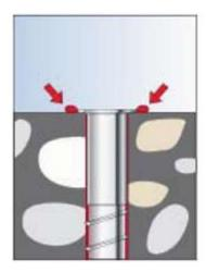
4. Make sure screw is flush with the surface and epoxy exits the top of the drill hole.
