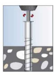
3. Screw the bolt into position.
