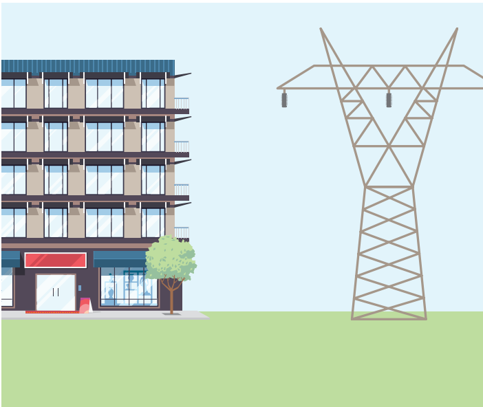
A building located at the edge of the ROW poses a high risk of induction as the upper levels of the building are closer to the power line.
