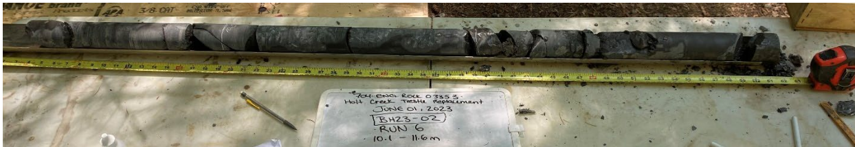
BH23-02 Rock Core 10.1 m to 11.6 m
