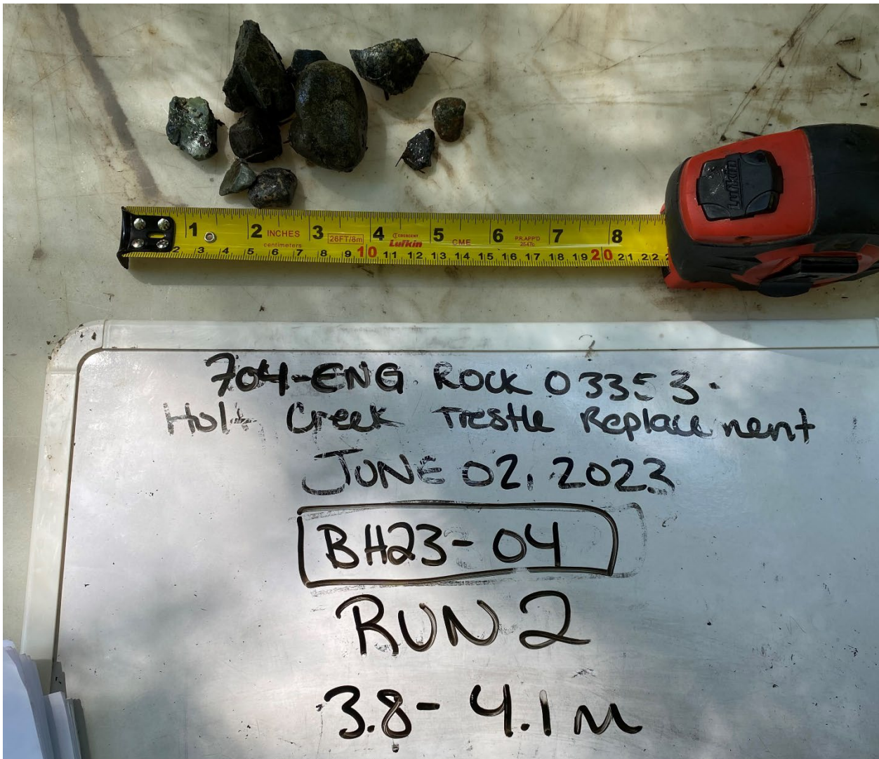
BH23-04 Rock Core 3.8 m to 4.1 m
