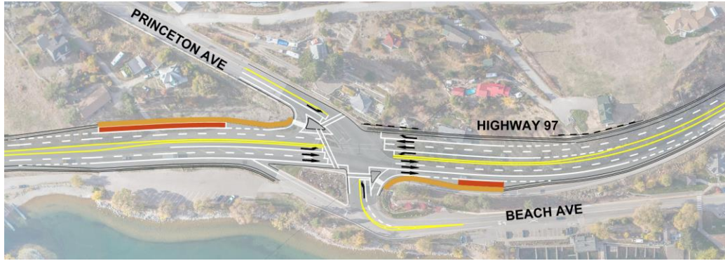
Figure 3.14: Princeton Avenue Intersection Transit and Safety Improvements – Potential Long-Term Layout with Option ER-A Implemented
