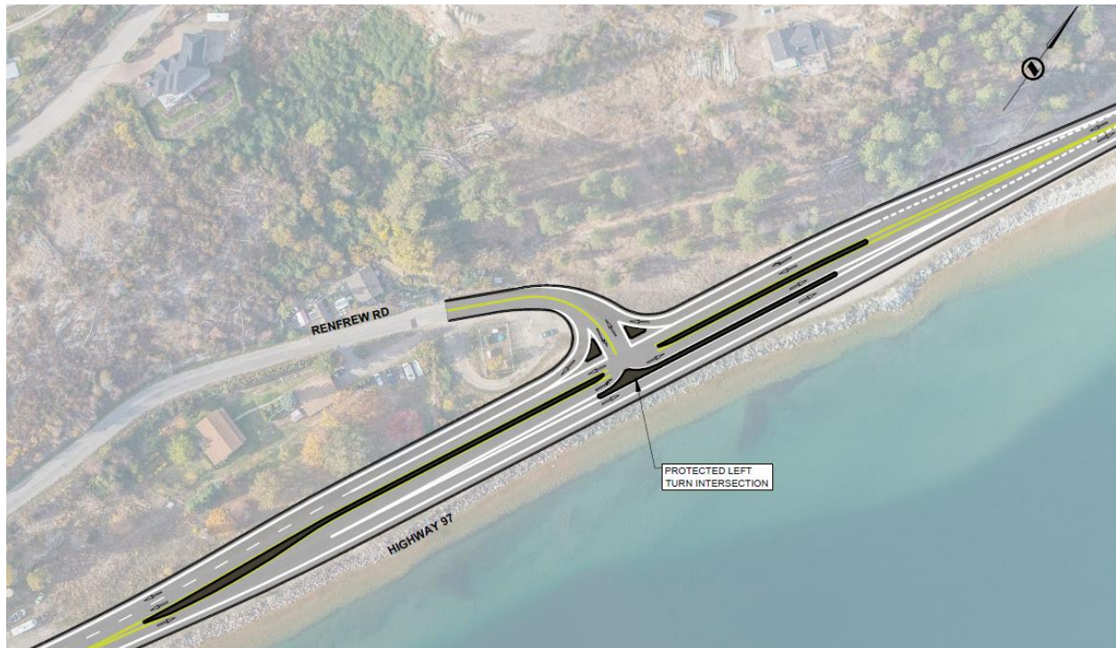
Figure 3.12: Renfrew Road Intersection Safety Improvements
