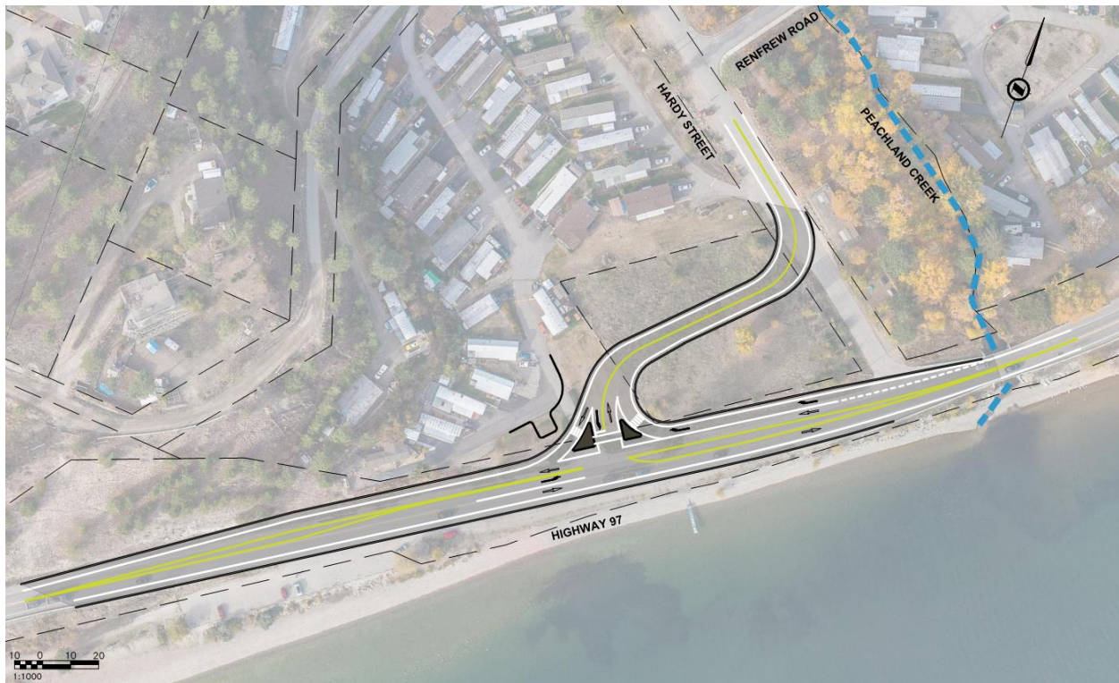
Figure 4.5: Hardy Street Intersection Safety Improvements
