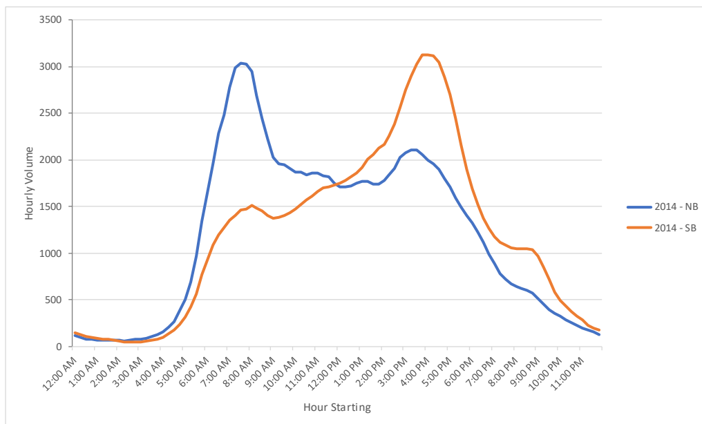
Figure A.1: Typical October weekday daily profile over the William R. Bennett Bridge
