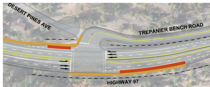
Figure 3.13: Trepanier Bench Road Signalization and Access Management Upgrades – Potential Long-Term Intersection Layout with Option ER-A Implemented
