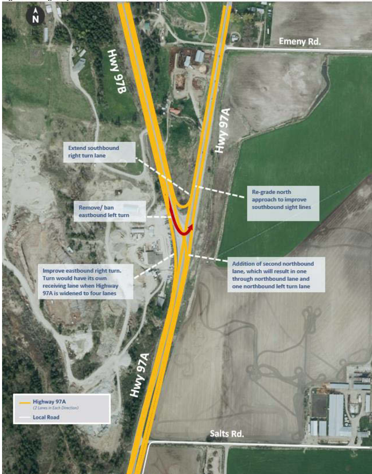
Figure 7-7: Highway 97A/B Junction At-Grade Improvements
