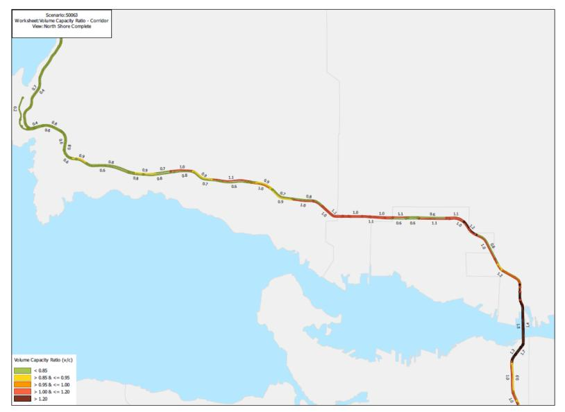
Figure 2.24: 2050 PM Peak Hour Corridor Volume-to-Capacity Ratios
