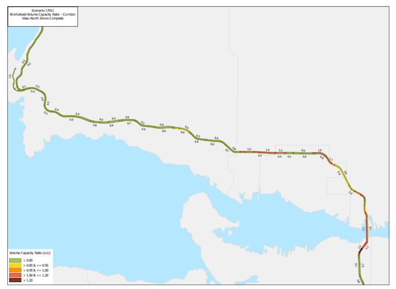
Figure 2.21: 2017 AM Peak Hour Corridor Volume-to-Capacity Ratios
