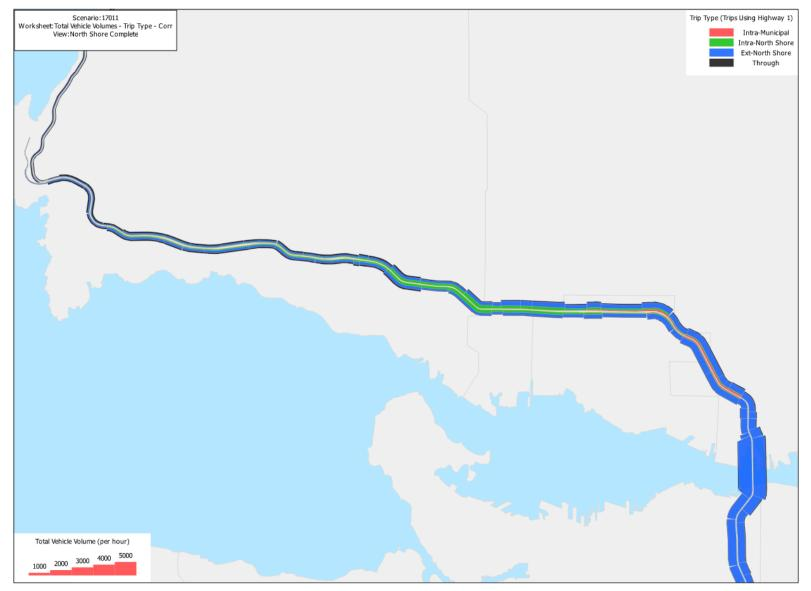
Figure 2.31: 2017 AM Peak Hour Trip Type Disaggregation
