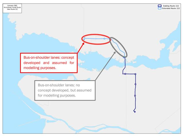
Figure 3.3: Infrastructure Concept for Extension of Route 222 Service on Highway 1 Using Bus-on-Shoulder System FOR DISCUSSION PURPOSES ONLY
