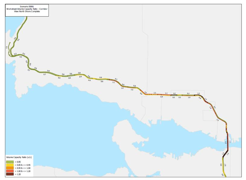
Figure 2.23: 2050 AM Peak Hour Corridor Volume-to-Capacity Ratios
