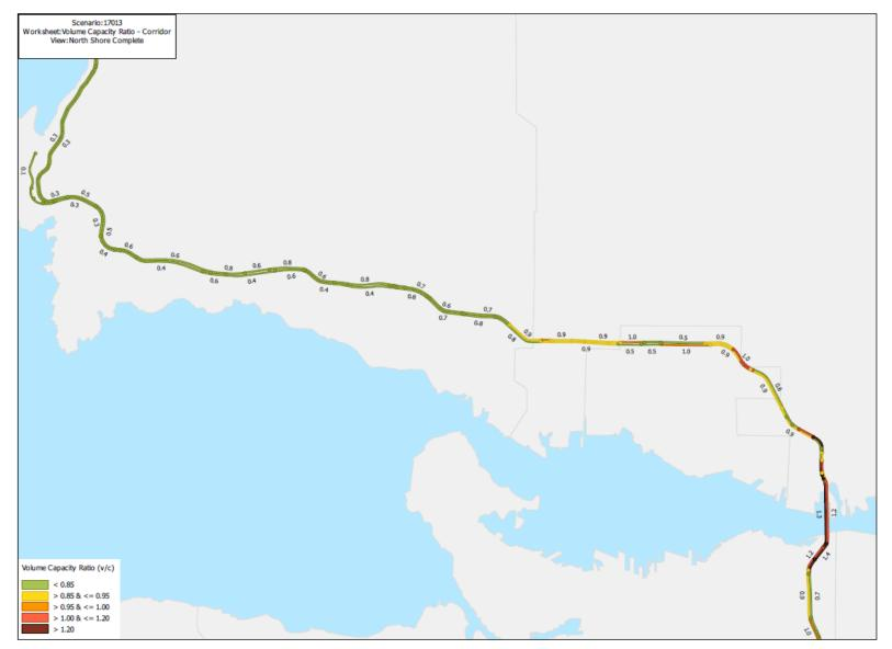
Figure 2.22: 2017 PM Peak Hour Corridor Volume-to-Capacity Ratios
