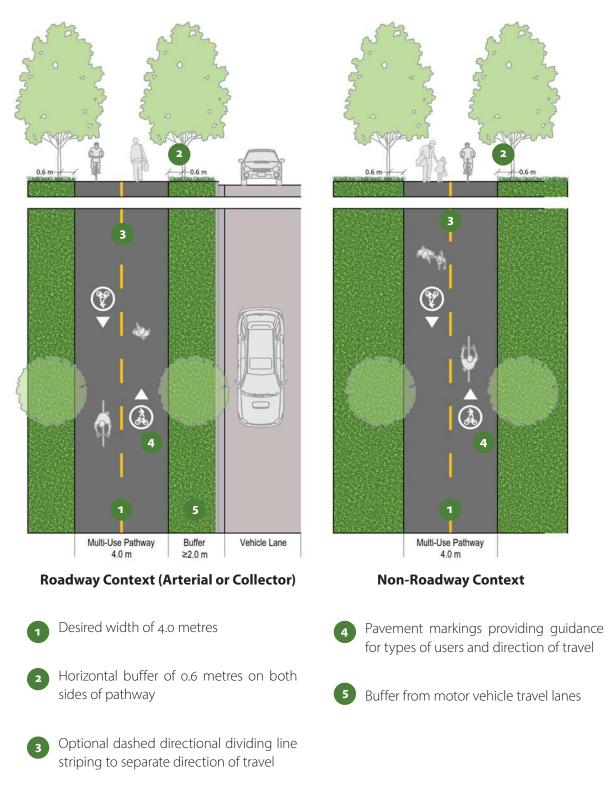
FIGURE E-58 // MULTI-USE PATHWAY CROSS-SECTION - DESIRED WIDTHS AND KEY FEATURES
