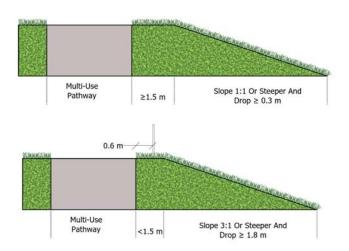
FIGURE E-61 // SIDE SLOPE OF GREATER THAN 1:3 AND A DROP OFF GREATER THAN OR EQUAL TO 1.8 METRES, TO A HAZARD (SUCH AS A WATER BODY) Source: Adapted from Trails in Alberta Highway Rights-of-Way, Figure 4.3
