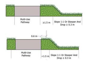
Figure E-59 // Side slope of greater than 1:1 and a drop off greater than or equal to  $0.3\ \text{metr3s}$
