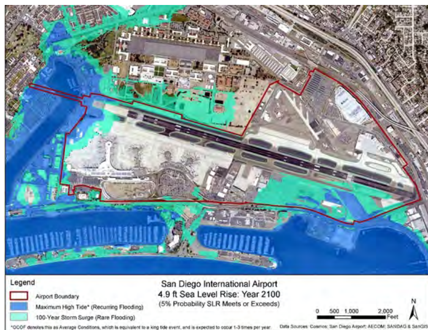
FIGURE 3-6 San Diego International Airport flooding forecast due to sea level rise, maximum high tide, and 100-year storm surge. 24
