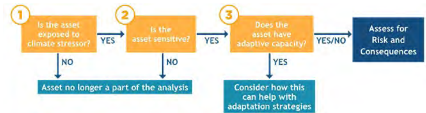
FIGURE 3-5 Steps for the vulnerability assessment conducted by the San Diego International Airport. 22
