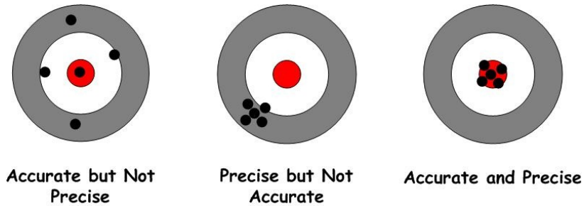
Figure 3.2: Dartboard Analogy - Definition of Precision and Accuracy
