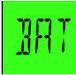
If the Alco-Sensor FST® does not have sufficient battery power to perform a test, either the display will not power on or **BAT** will be displayed and testing will be disabled. The battery strength indicator has three bars
