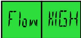
**Flow HIGH** indicates that the subject's breath flow exceeded the maximum allowable flow rate.
