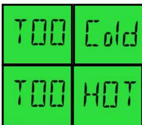
Device temperature **TOO Cold** for test type being performed.
