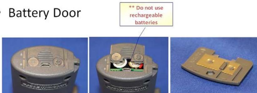
**Batteries** - The battery cover is located on the base of the Alco-Sensor FST®. Two AA alkaline batteries should run well in excess of 1000 tests at room temperature. The device is reverse-polarity protected. Rechargeable batteries are not to be used.
