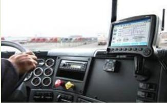
Mobile data terminals are non-hand-held computerized devices without a telephone function that are licensed through Industry Canada under the *Radiocommunication Act* (Canada). These devices are used exclusively to communicate with a dispatcher or control centre and where pre-packaged data are transmitted, point in time, over a set radio frequency.
