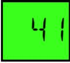
Digital results will be displayed for concentrations from 0 to 59 mg%. In this example, the result is 41.
