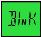
An air blank test (**BLNK**) is run automatically by the device to ensure that there is no alcohol present from a previous test.
