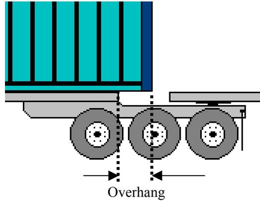
**Comments:** The overhang is measured from the rear of the deck or cargo carrying area of the lead semitrailer on B Trains (not from the extended frame which supports the fifth wheel).
