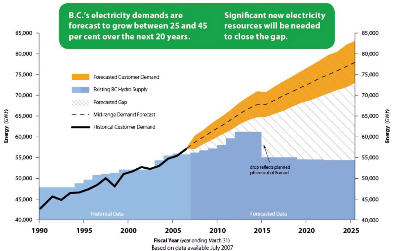
Figure 4: Forecast of energy shortfall for the province of British Columbia (BC Hydro, 2008).
