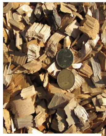
Wood chips for biomass heating
