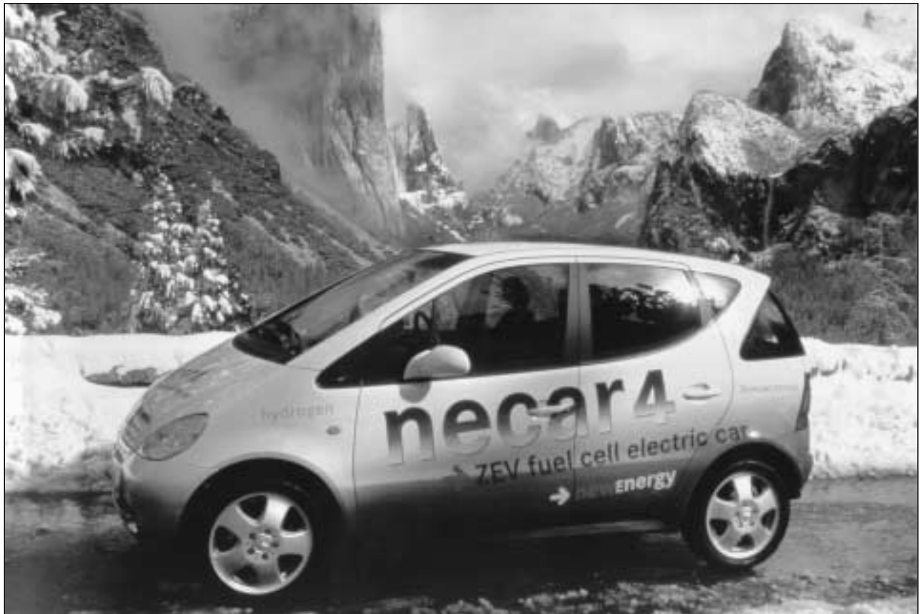
NECAR 4 — powered by a Ballard fuel cell and emitting only water vapour
