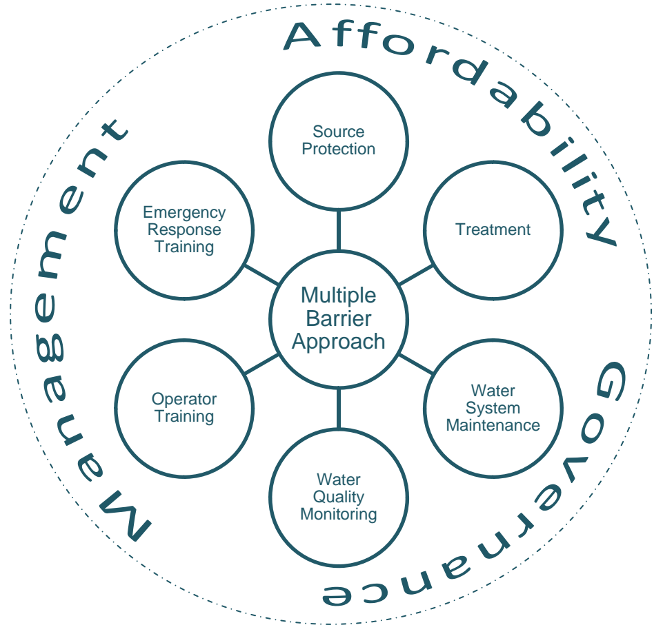
Figure 1-2. Multiple Barrier System of Drinking Water Protection
