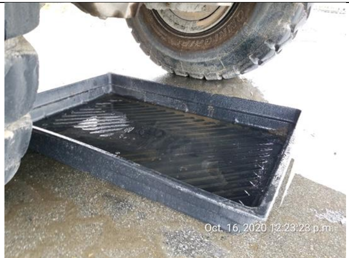
Photo 12. Secondary containments and drip trays should be inspected to remove quantities of accumulated rainwater.
