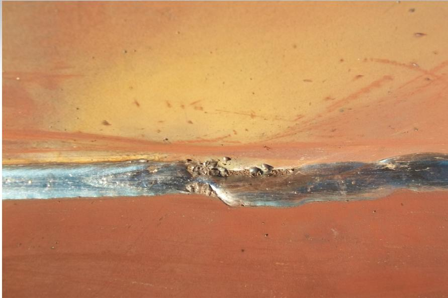
Incorrect profile and out of line weld
