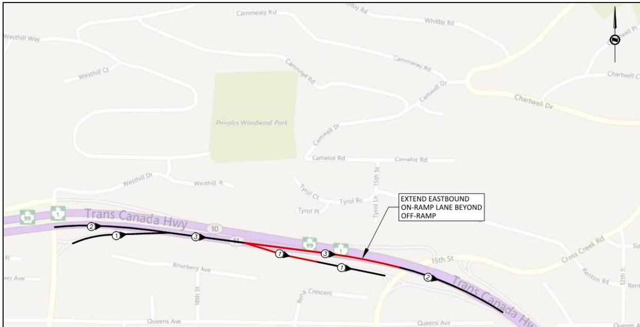
Figure 4.11: 21st Street Eastbound On-Ramp Extension (shown in red)
