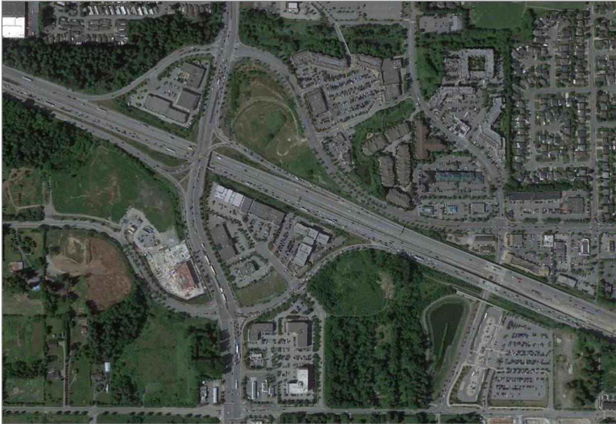
Figure 3.4: Median Ramp Configuration (Right) and Separate General-Purpose Interchange (Left)
