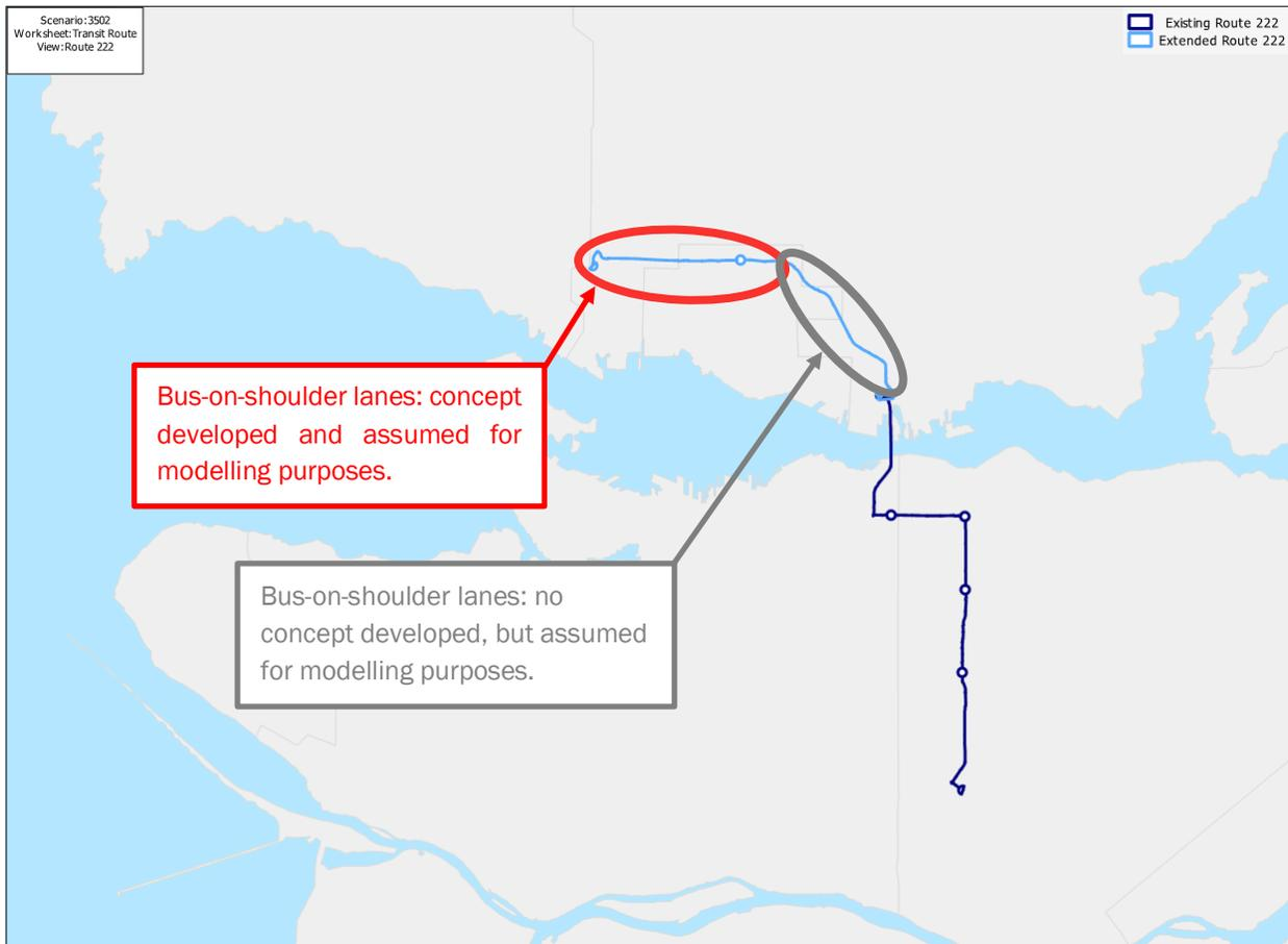
Figure 3.3: Infrastructure Concept for Extension of Route 222 Service on Highway 1 Using Bus-on-Shoulder System
