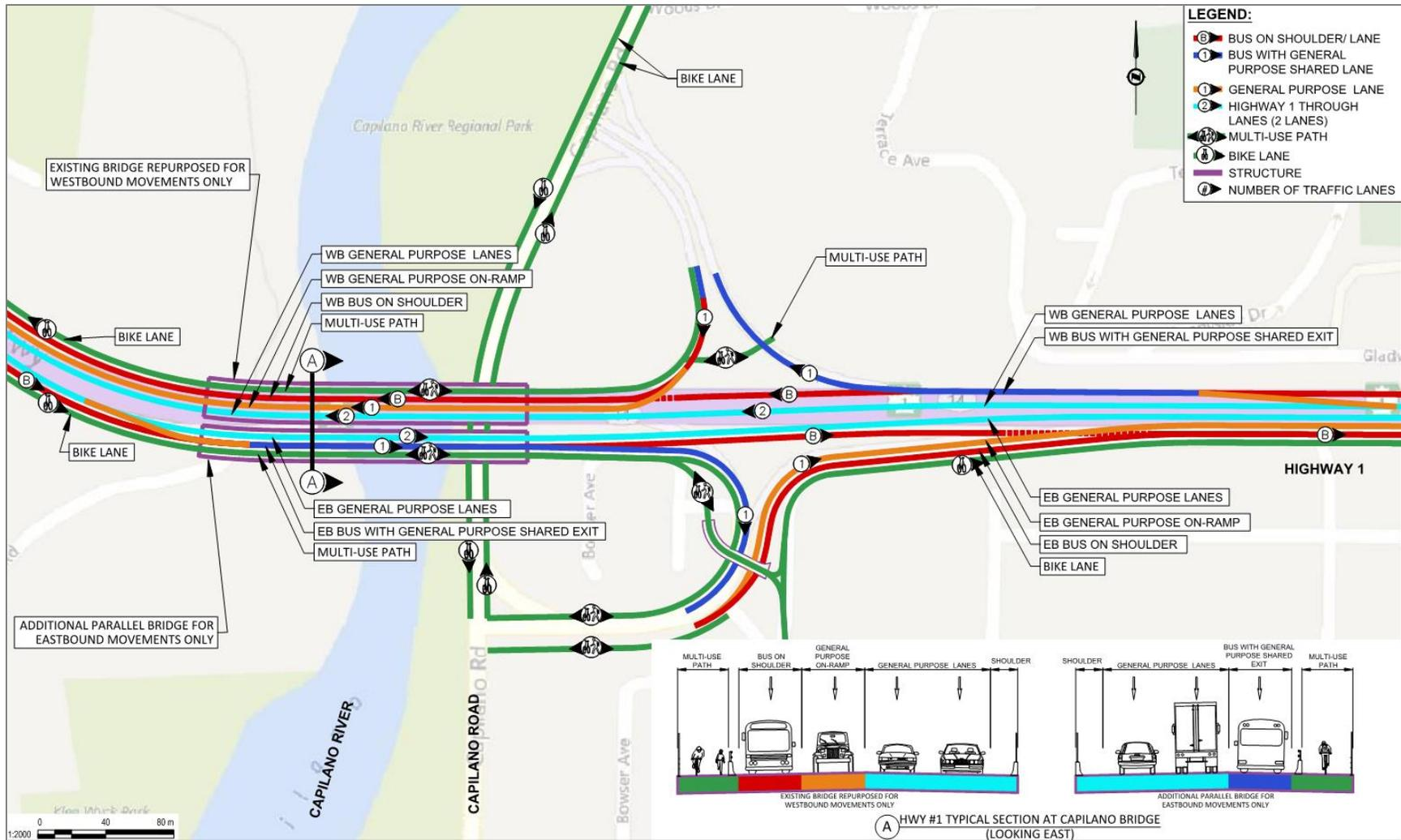
Figure 4.3: Capilano Road Interchange Concept - New South Bridge
