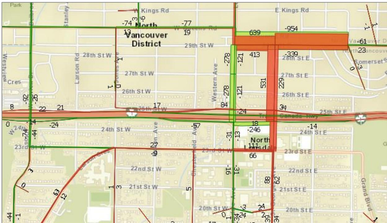
Figure 4.14: 2050 AM Peak Hour Volume Differences with St. Georges Avenue Overpass Improvements
