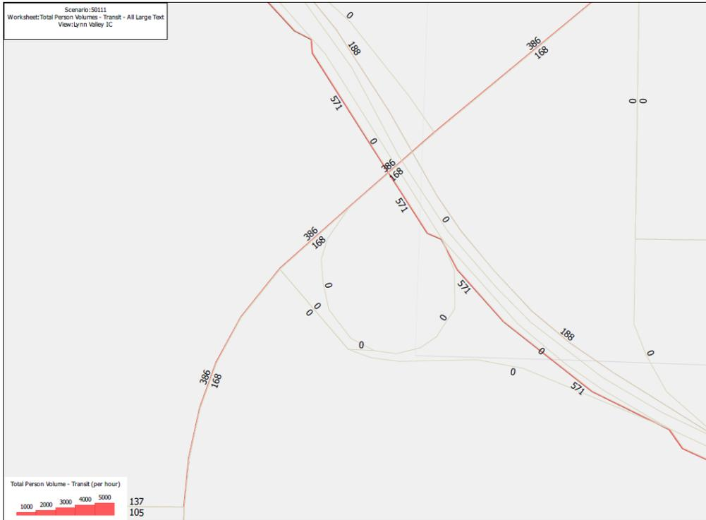
Figure 4.6: Lynn Valley Interchange Transit Volumes (2050 AM Peak Hour; with Basic Bus-on-Shoulder Concept)
