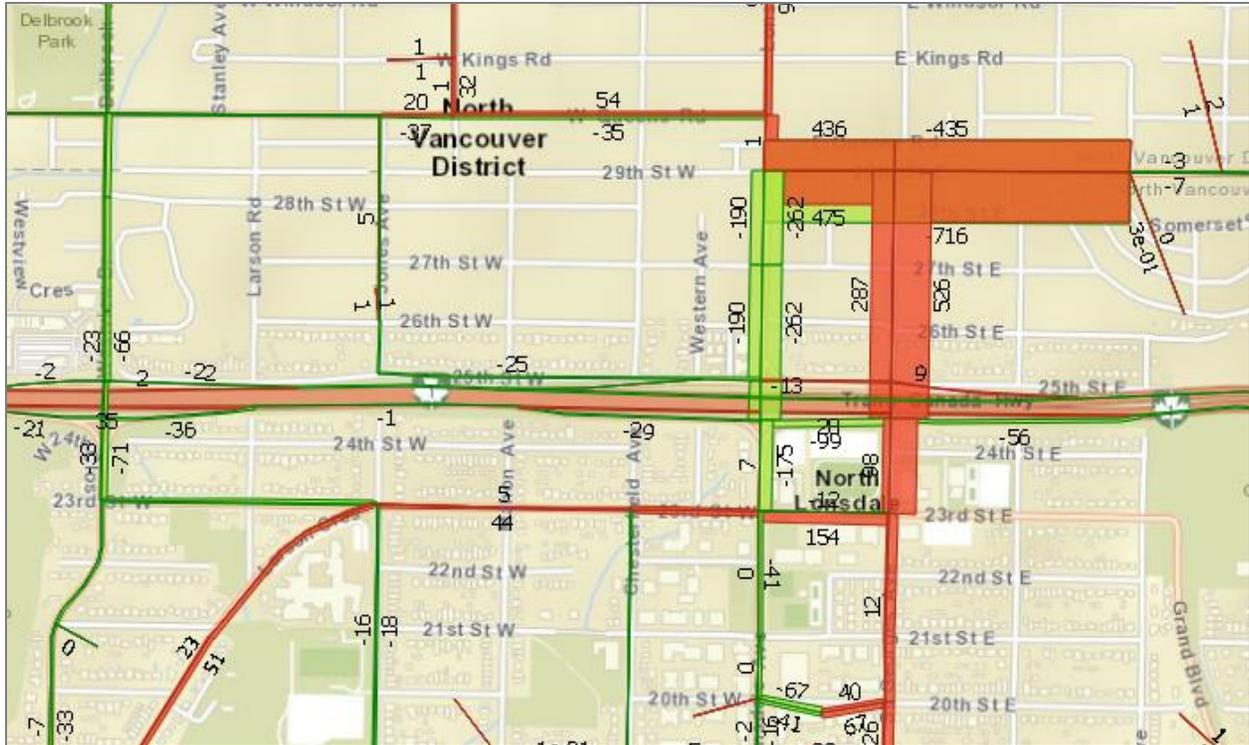
Figure 4.15: 2050 PM Peak Hour Volume Differences with St. Georges Avenue Overpass Improvements
