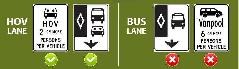
A diamond symbolizes a "reserved lane." It can be used for bus lanes, HOV lanes, or bicycle lanes and must be combined with either a passenger vehicle, van, bus or bicycle symbol to dictate the intended use of the lane. A stand-alone diamond symbol does not necessarily mean an HOV lane.
