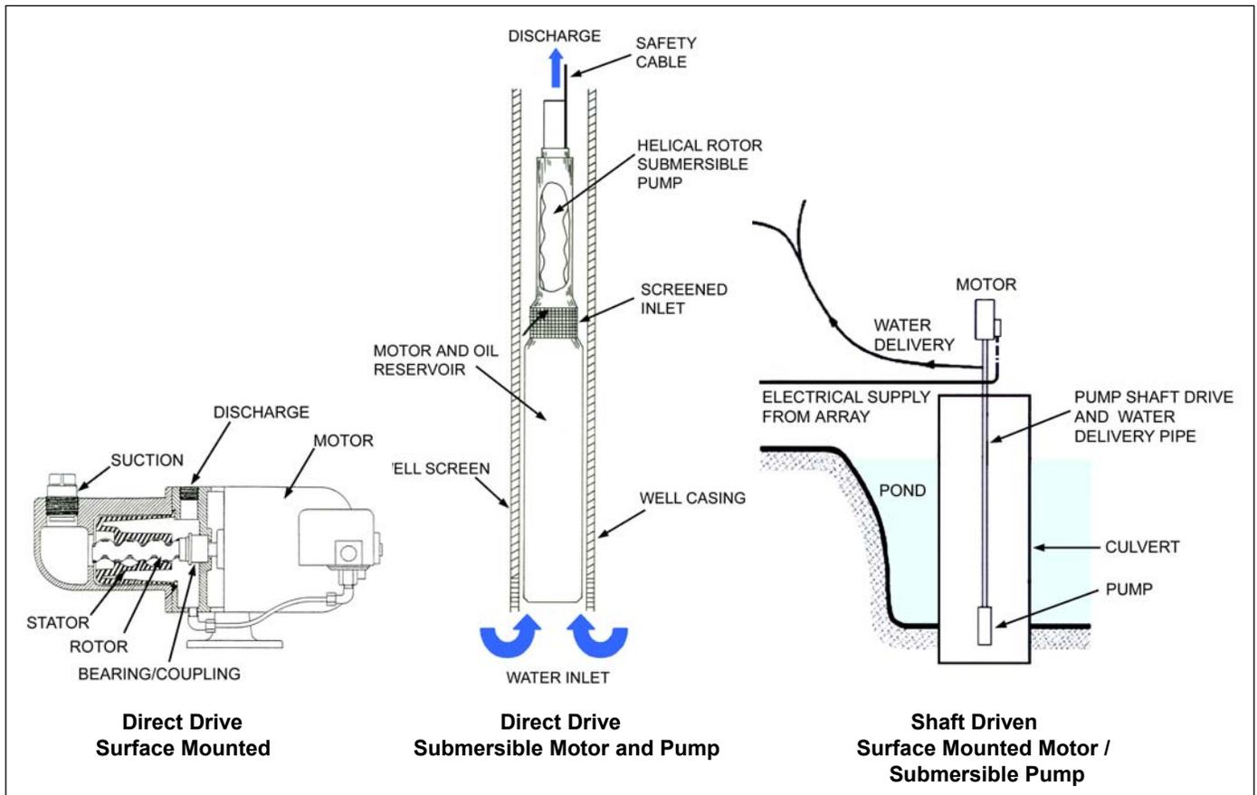
Figure 4 Progressive Cavity Pump Drive Options
