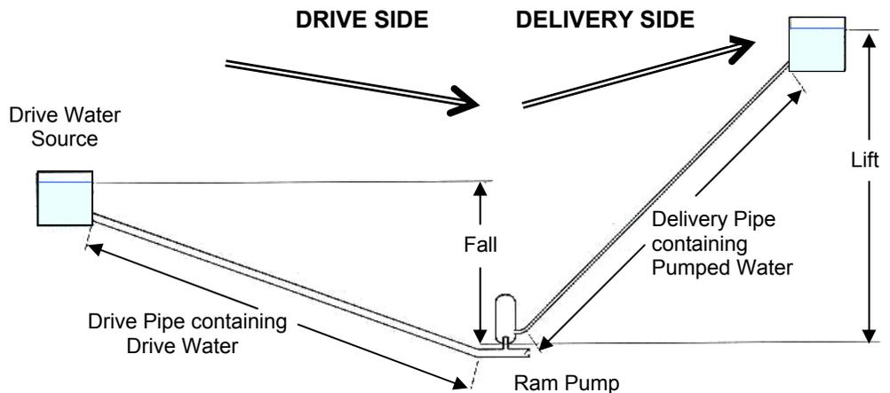
**Figure 9 Hydraulic Ram Pump**
