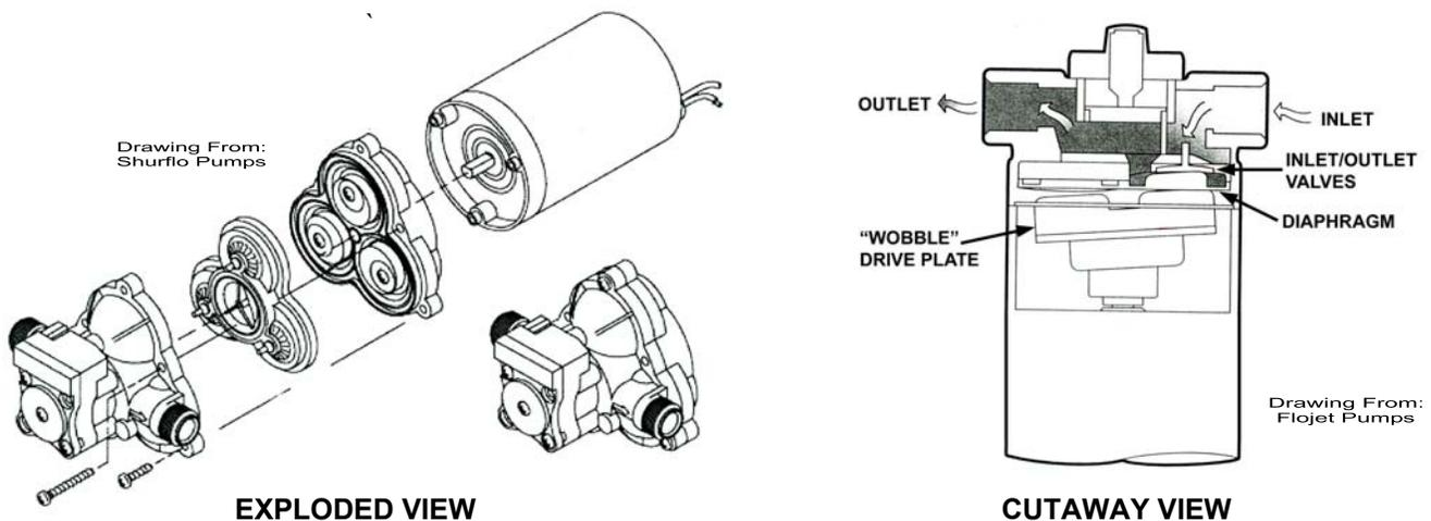
**Figure 3 Typical Diaphragm Pump**
