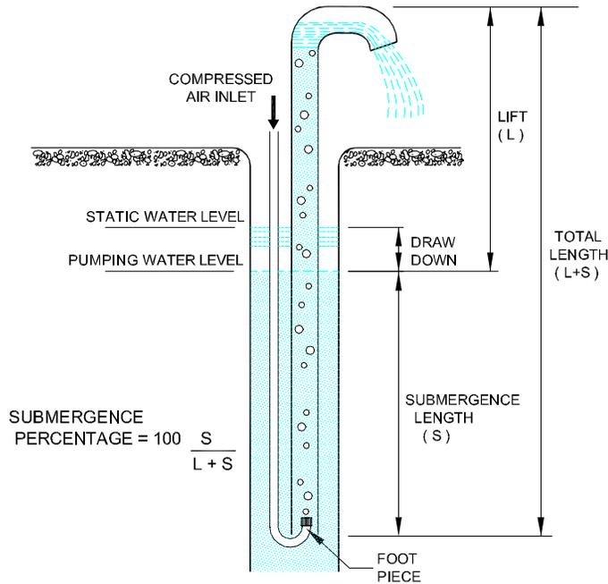
**Figure 8 Air Lift Pump**
