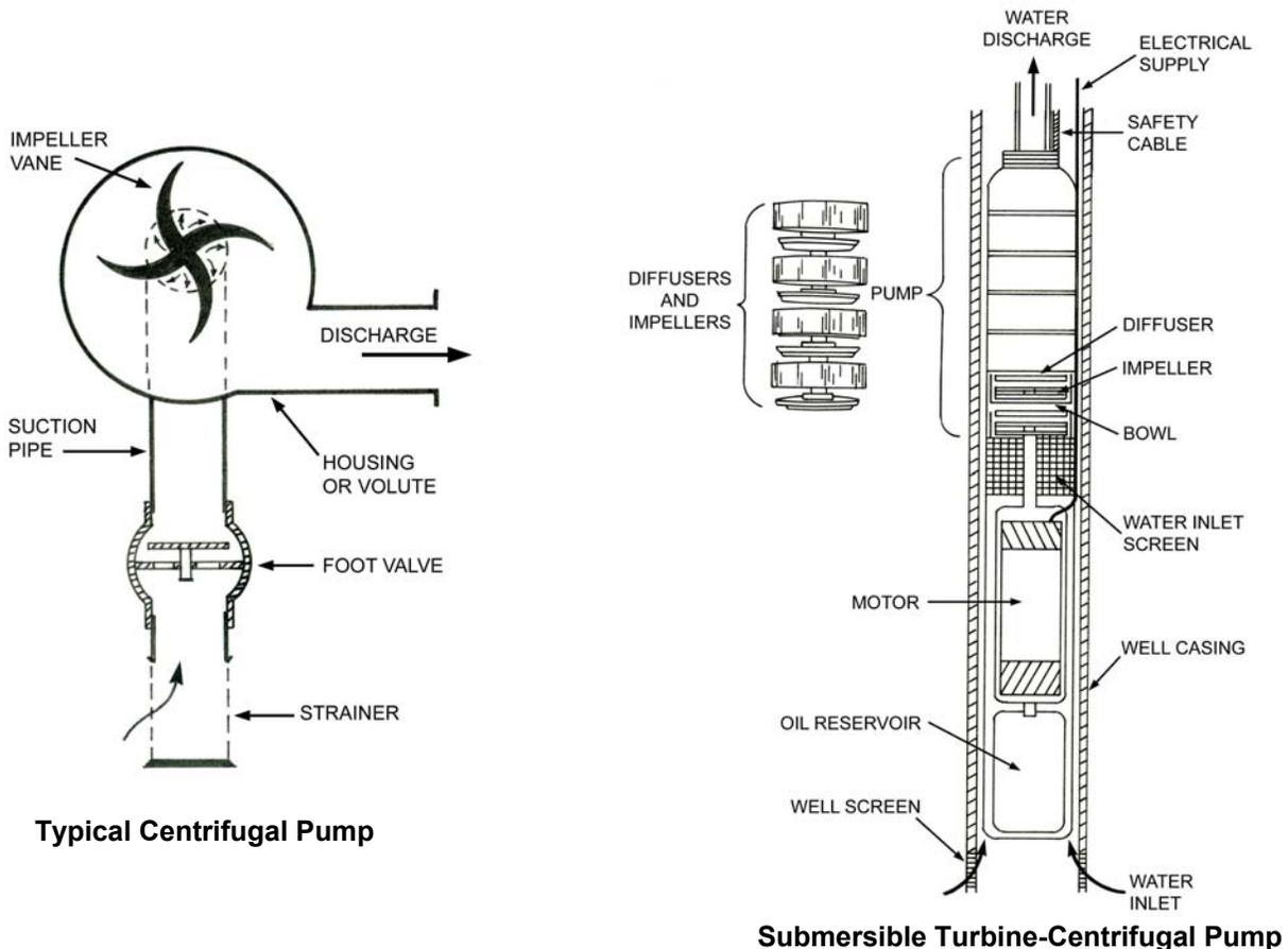
**Figure 6** Cutaway of Centrifugal Pumps
