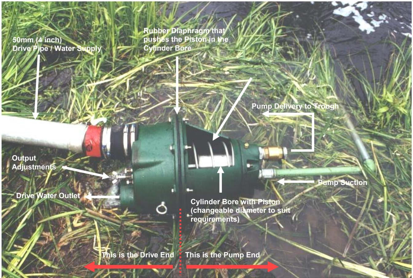
**Figure 10**      **Modified Hydraulic Ram Pump (*Glockemann 320*)**      (delivery line not shown)
