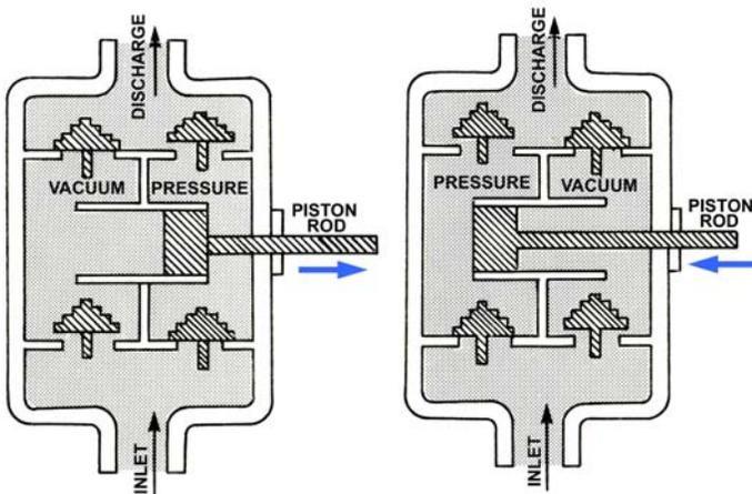
**Figure 2 Double-Acting Piston Pump**
