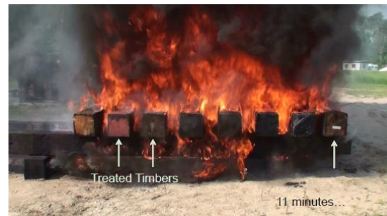
Figures 1. Point source ignition cross beam tests showing “exponential rate of spread” (Bridge Timber Protection, Thomasson 2013).
