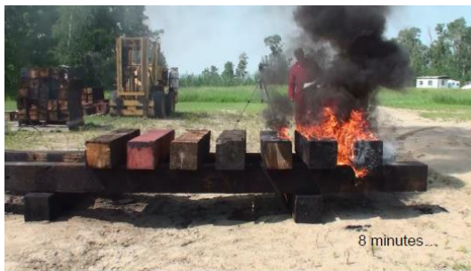
Figures 1. Point source ignition cross beam tests showing “exponential rate of spread” (Bridge Timber Protection, Thomasson 2013).
