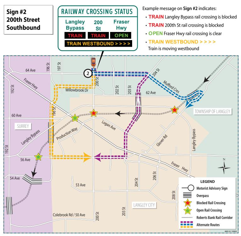
Driving southbound on 200th St, drivers will see Sign #2. Based on the example message on Sign #2, drivers can choose alternate routes to avoid waiting at the blocked rail crossings ahead.
