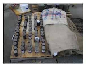
Figure 10: Example of damp burlap sacks being used to keep grout sample cylinders cool and moist.
