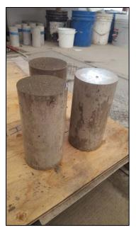
Figure 1: Ministry Standard 2" test cylinders.
