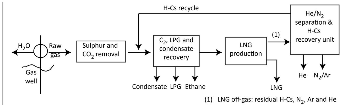
Figure 3. A liquefied natural gas (LNG) train with helium (and other byproduct) recovery (after Clarke and Van Schagen, 2010).
