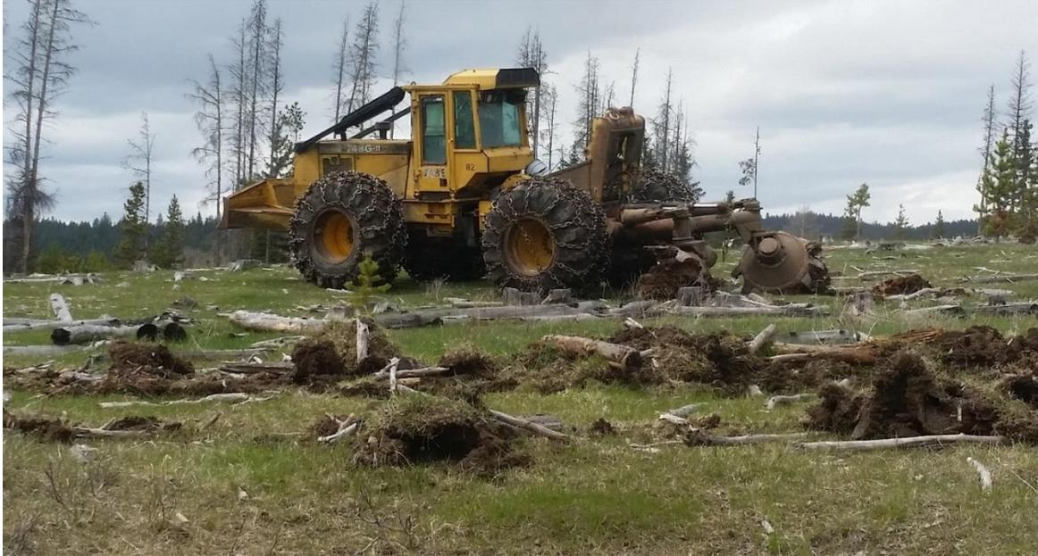
Photo 15. Example of poor disturbance on single pass disc trenching. Note the flat, compact soils which are very difficult to provide adequate disturbance. Photo provided by Clayton Franz
