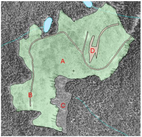
The image above shows the how the 3 strips that were greater than 20m wide, and less than 20m apart were lumped into a single stratum.
