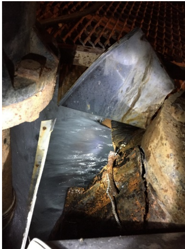
Photo 9: View of rupture in bypass pipe associated with the tunnel diverting water from the head pond of the Spillimacheen dam.
