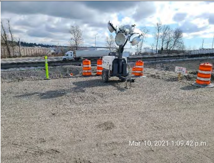
Photo 35. Example of stationary equipment lacking a drip tray.
