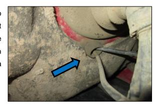
Locate a good vehicle ground point for radio power connections. Connect the negative (-) lead to a central grounding point close to the battery. Do not connect the radio ground wire directly to the negative (-) battery post. If a central grounding point is unavailable, a vehicle frame grounding point provides the next best low resistance ground. Use a ring lug crimped to the stripped wire end and a self-tapping screw or existing bolt to connect the ground wire.
