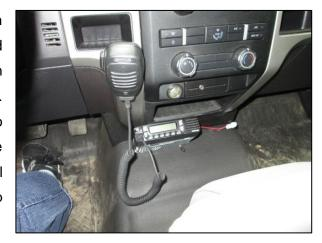
Ambient vehicle and road noise can make it hard to hear your radio. Install an external speaker so that
