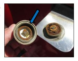
Ensure that the antenna connector at the back of the radio is tight, and that the cable is not kinked at this connection.
