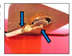
Ensure that the antenna is screwed properly to the base and is sealed from moisture by a rubber O-ring (arrow points to where an O-ring is missing). If the O-ring is missing or this connection loose, the antenna-to-base contact may become corroded.
