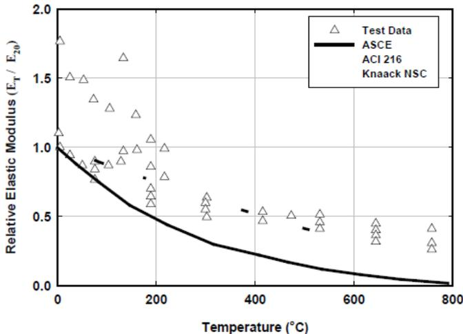
Figure 15 Variation of elastic modulus for normal strength concretes.
