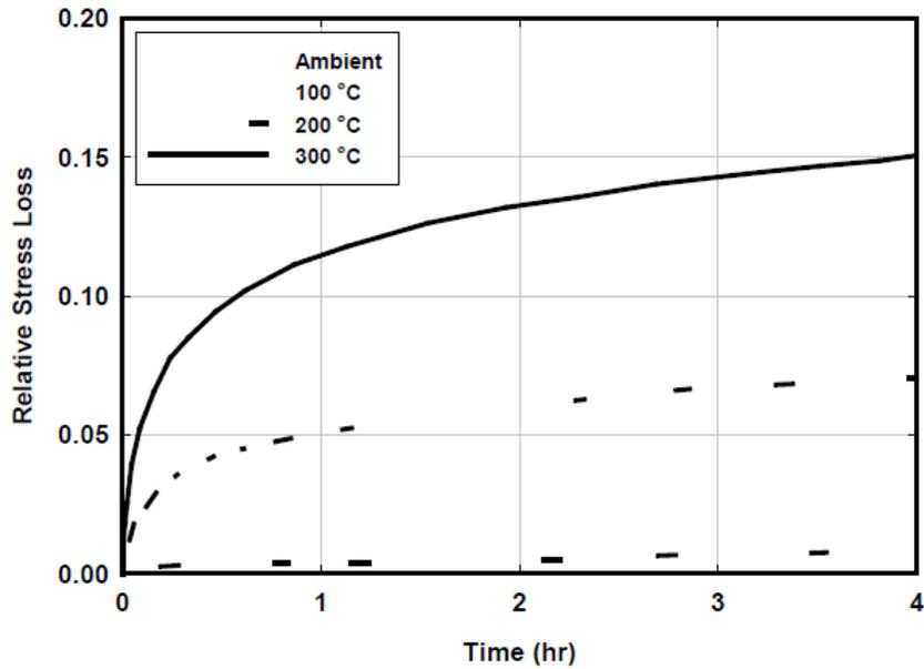
Figure 26 Stress loss over time for strands heated to various temperatures after being pretensioned to 70% of the tensile strength ( $0.7 f_{pu}$ ). At temperatures above  $300^{\circ}\text{C}$  the strands failed.
