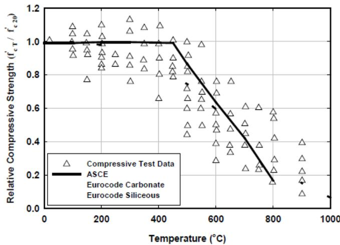
Figure 13 High temperature compressive strength of normal strength concrete.
