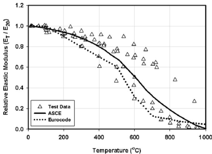
Figure 7 Reduction in elastic modulus of structural steel at high temperatures
