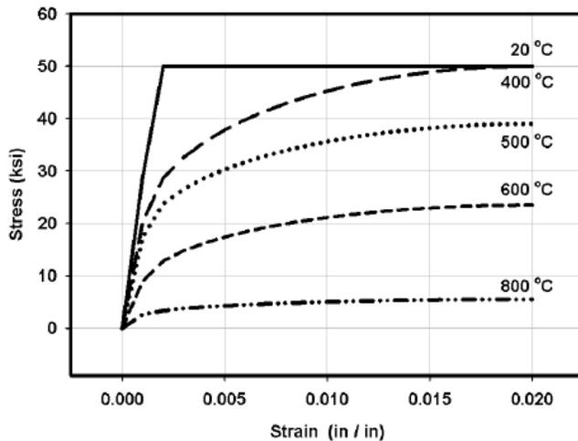
Figure 8 Change in shape of the stress-strain curve for Grade 50 steel based on the Eurocode model.
