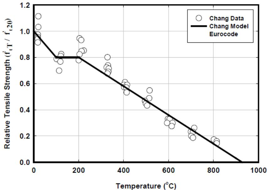
Figure 25 Post-fire tensile strength of concrete as a function of temperature.
