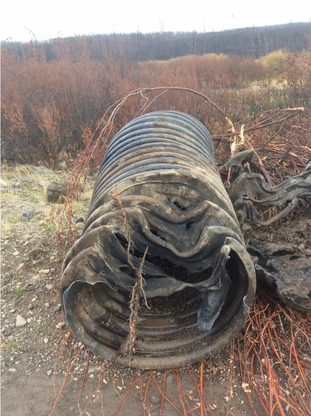
Photo 7b - Removed melted plastic culvert
