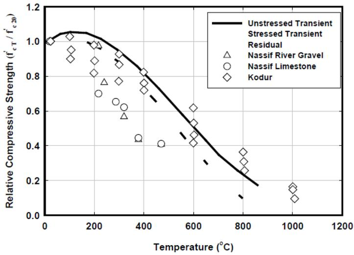
Figure 24 Post fire compressive strength of normal strength concrete.
