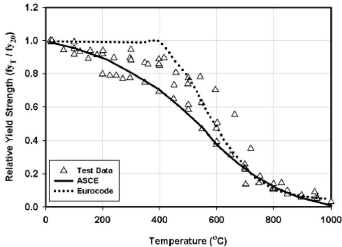
Figure 6 Reduction in yield strength of structural steel at high temperature.
