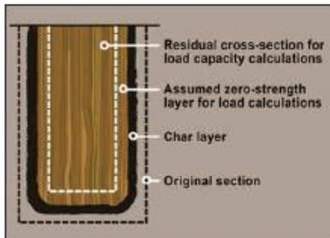
Figure 5—Reduced section approach to fire-damaged wood.
