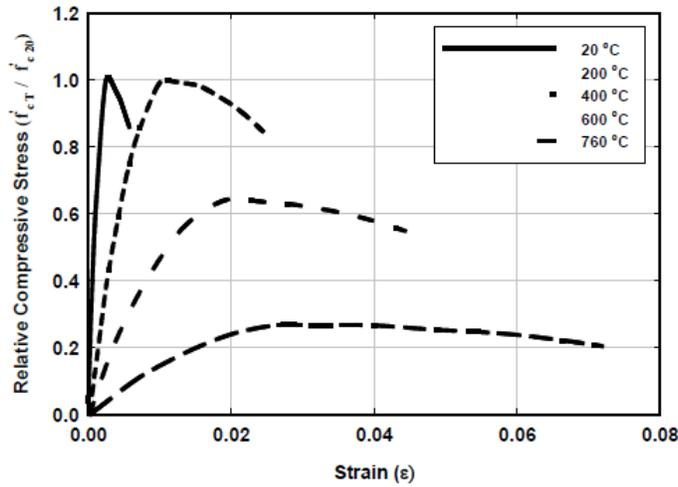
Figure 16 ASCE temperature-dependent stress-strain models.
