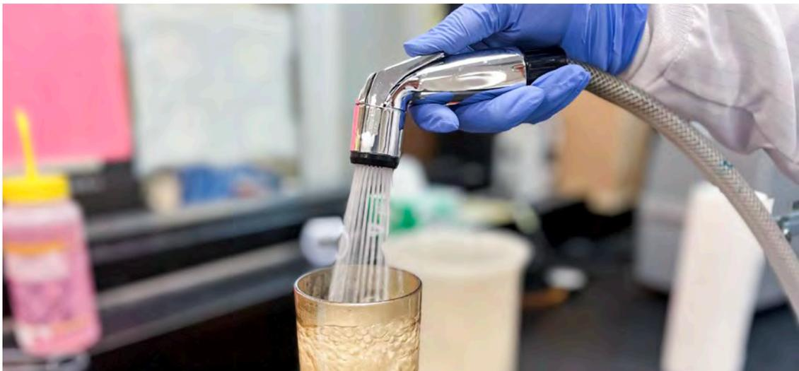
A Laboratory Technologist from the BC Centre for Disease Control Public Health Laboratory is processing drinking water using the membrane filtration technique. This is a provincially approved testing method for drinking water microbiological analysis. Quality assurance practices, such as aseptic technique, buffer washes, and other quality control measures are required to ensure test result reliability.
