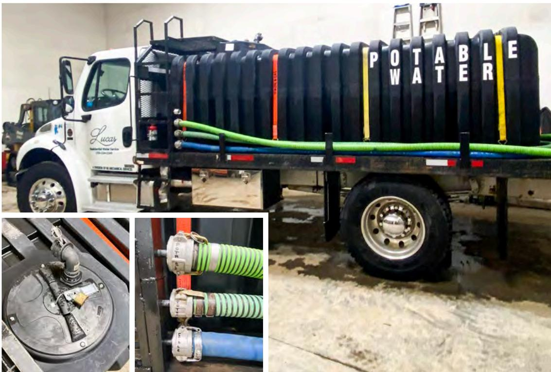
(Above) Northern Health inspecting a bulk water hauler operating out of Charlie Lake (Peace River Regional District). (Left) Lockable access hatch to the potable water tank for monitoring and filling the tank. (Right) Hoses labelled to indicate they are to be used only with potable water. Nozzles are also attached to a connection point to prevent contamination.
