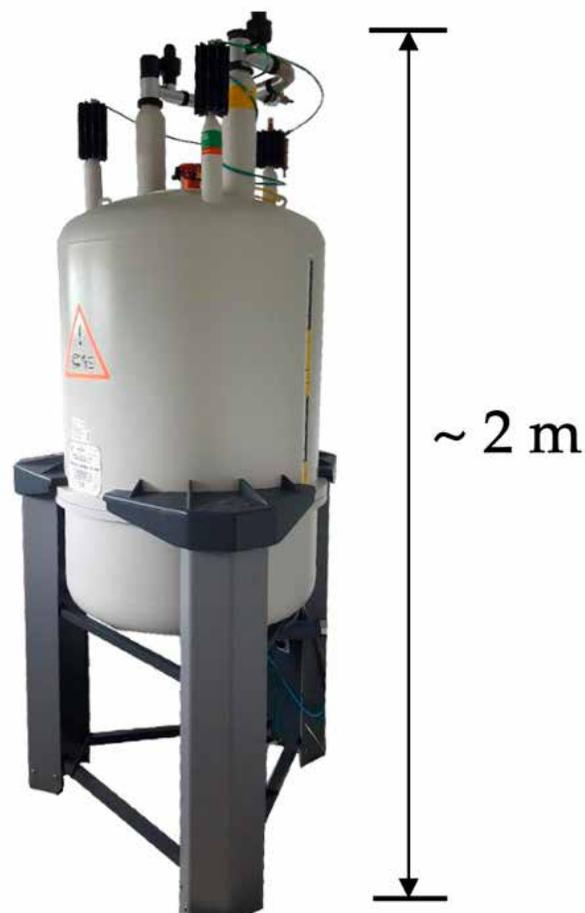
Figure 1. MRI scanner with 11.74 T magnetic field strength. Sample is lowered to the center of the cylinder from the top using an airlift. Magnetic field is created by a current running in a loop of superconducting material cooled using liquid helium (4 Kelvin,  $-269^{\circ}\text{C}$ ). Helium evaporation is minimized with nitrogen (77 Kelvin,  $-196^{\circ}\text{C}$ ) surrounding the helium.
