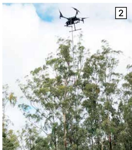
Figure 3. Seed collected with the DeLeaves during a test flight in a eucalypt seed orchard (Mike Sutton (left) and Tim Hitchens (drone pilot, right)). Credit: Mike Sutton, Forestry Corporation of NSW.
