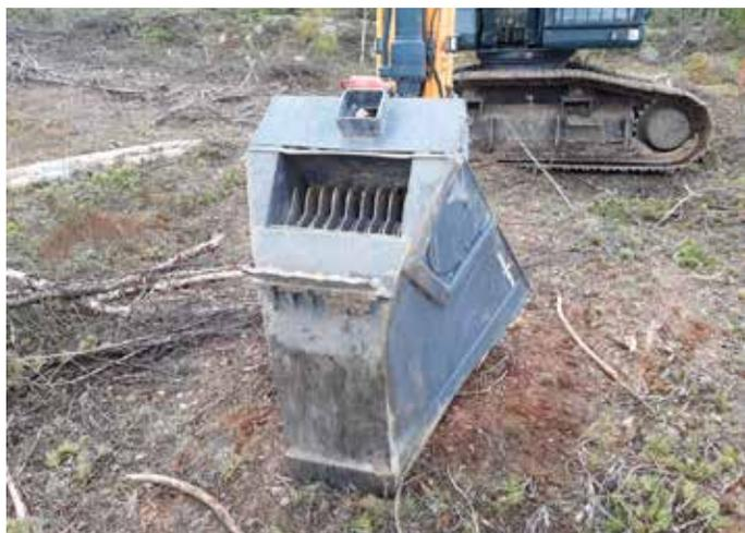
Figure 1. Improved version of the direct seeding bucket (DSB) equipped with a separate scarification blade.
